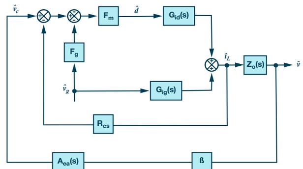
Figure 9. Current-mode buck small signal diagram from input voltage to output.
