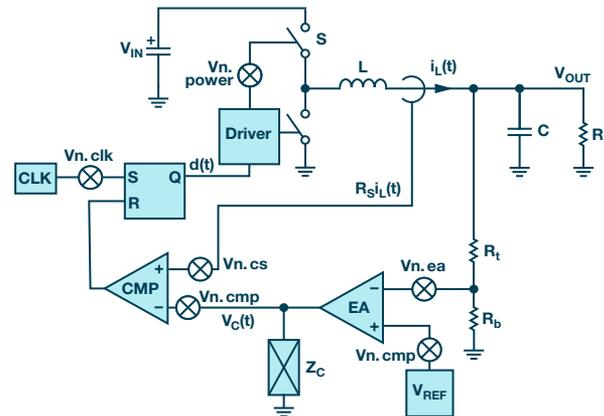
Figure 6. Typical current mode buck regulator control scheme.
