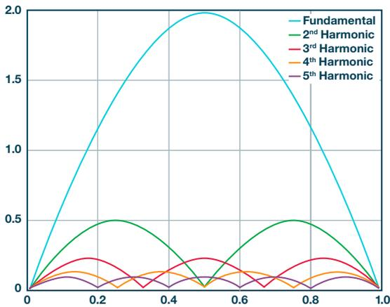
Figure 3. Buck regulator V<sub>OUT</sub> ripple amplitude vs. duty.
