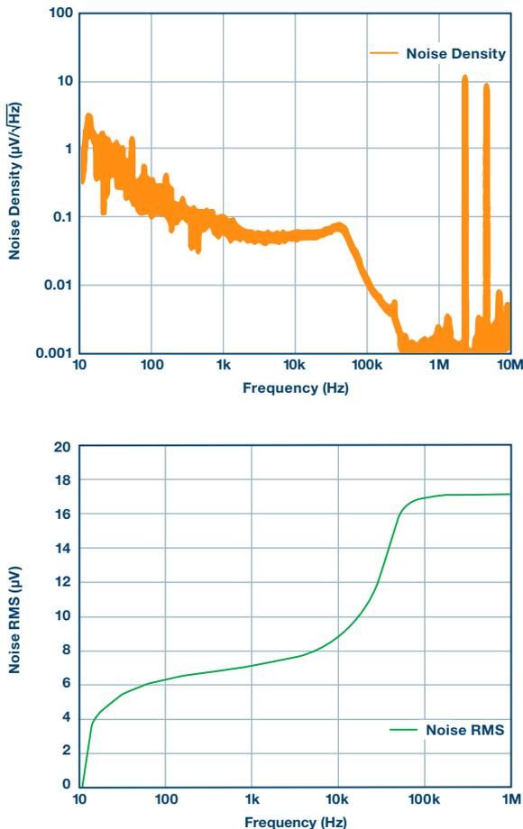
Figure 7. ADP5014 output noise performance with an additional LC filter.
