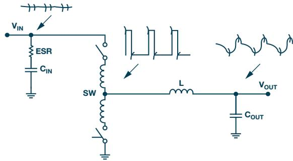
Figure 8. Buck regulator high frequency spike and ringing noise.
