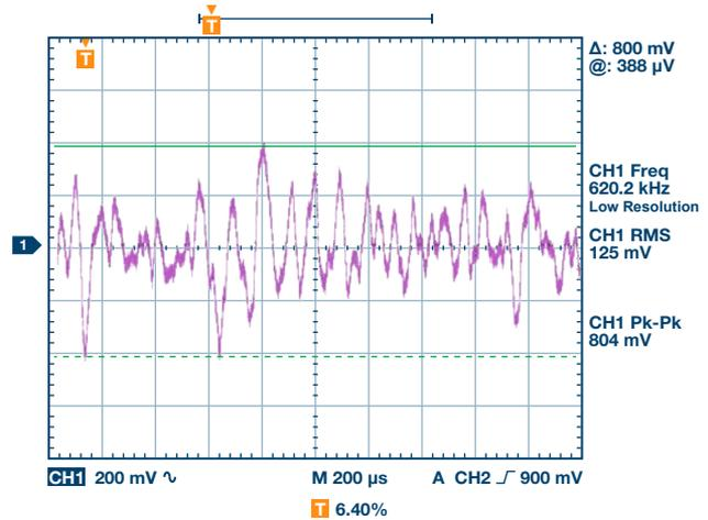
Figure 5. V<sub>OUT</sub> with an additional filter (using 1000× pre-amp to measure).
