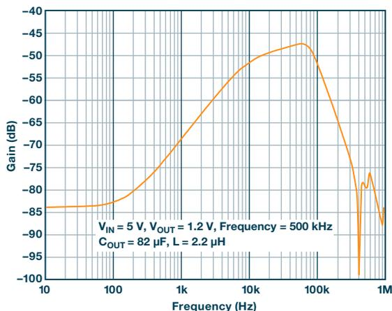
Figure 11. PSRR simulation by SIMPLIS mode.
