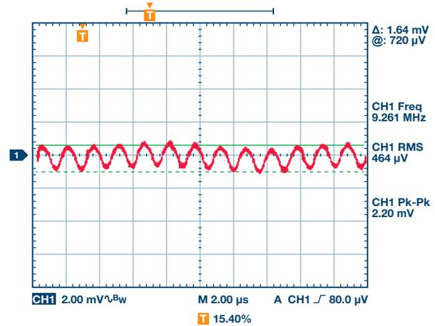
Figure 4. V<sub>OUT</sub> without an additional filter.
