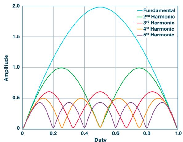
Figure 2. Buck regulator  $V_{SW}$  amplitude vs. duty.
