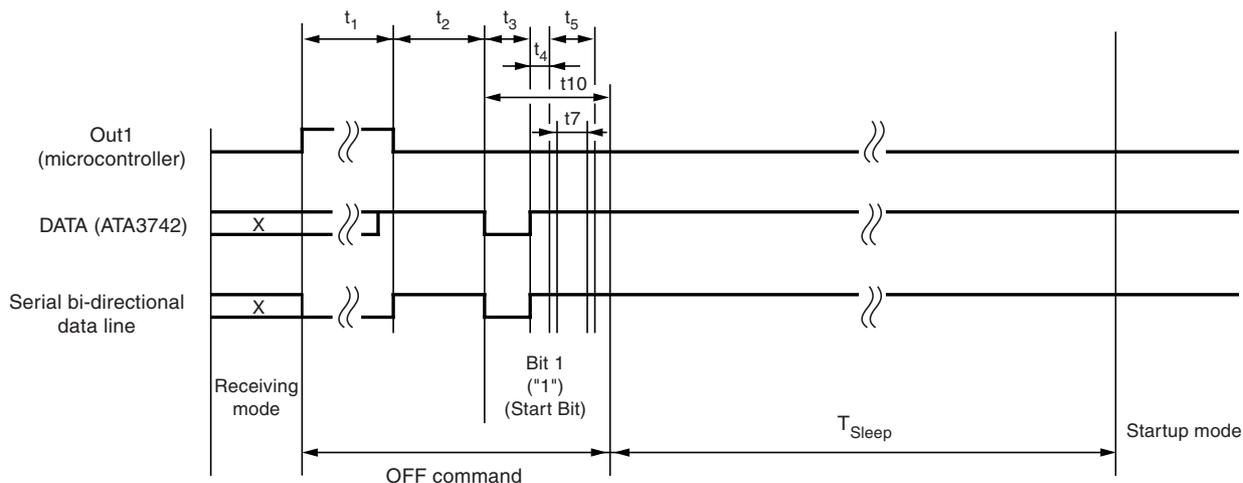
**Figure 5-12.** Timing Diagram of the OFF Command via Pin ENABLE
