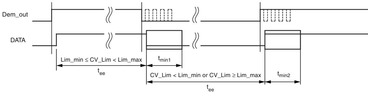
**Figure 5-10.** Steady L State Limited DATA Output Pattern after Transmission
