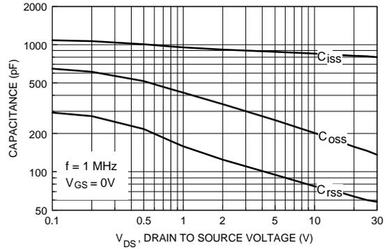
Figure 8. Capacitance Characteristics.
