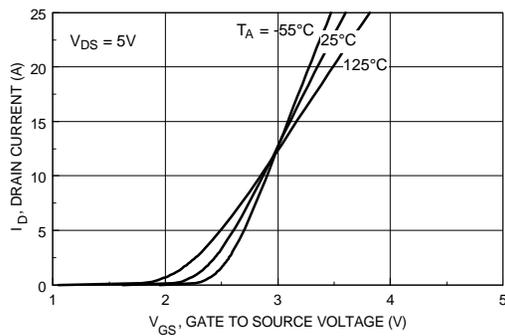
Figure 5. Transfer Characteristics.
