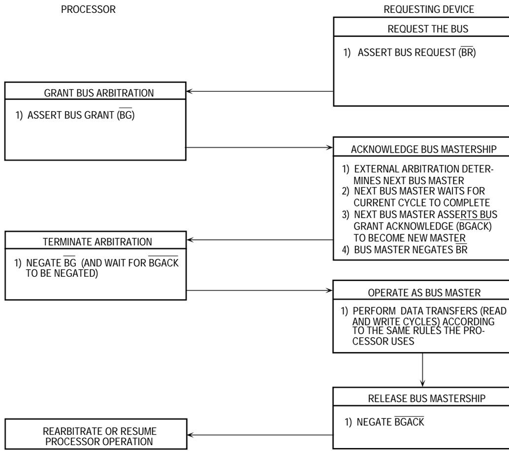
**Figure 5-13. 3-Wire Bus Arbitration Cycle Flowchart
