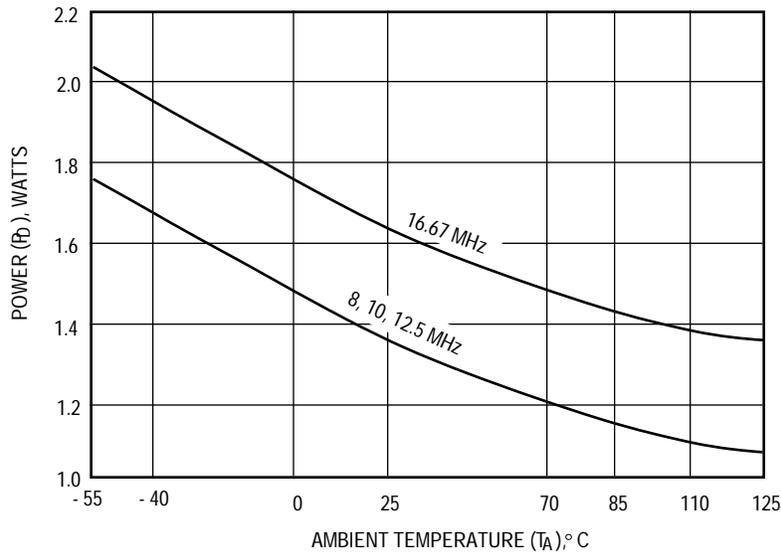
**Figure 10-1. MC68000 Power Dissipation (P<sub>D</sub>) vs Ambient Temperature (T<sub>A</sub>) (Not Applicable to MC68HC000/68HC001/68EC000)**
