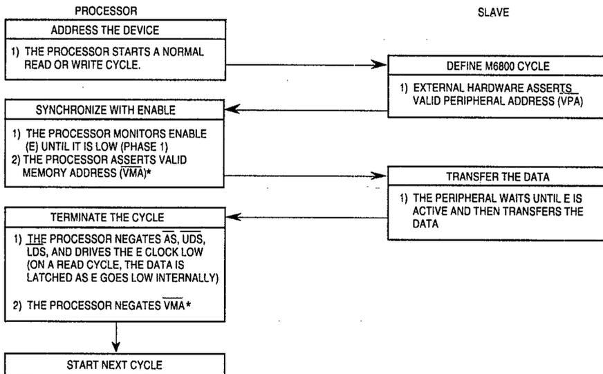
\* For MC68008-based systems,  $\overline{VMA}$  is supplied by external circuitry.
