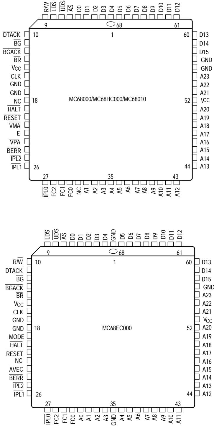
Figure 11-3. 68-Lead Quad Pack (1 of 2)
