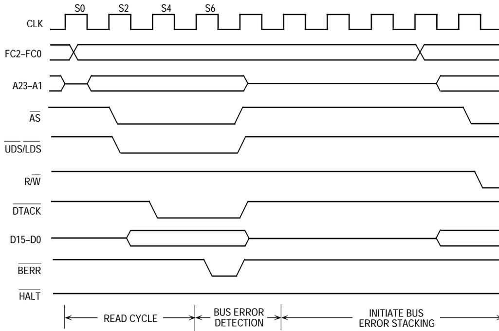
**Figure 5-26. Delayed Bus Error Timing Diagram (MC68010)**
