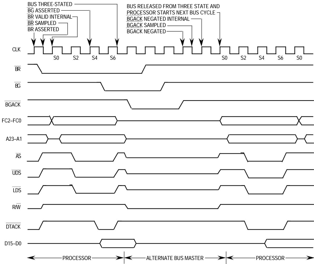
Figure 5-21. 3-Wire Bus Arbitration Timing Diagram—Special Case
