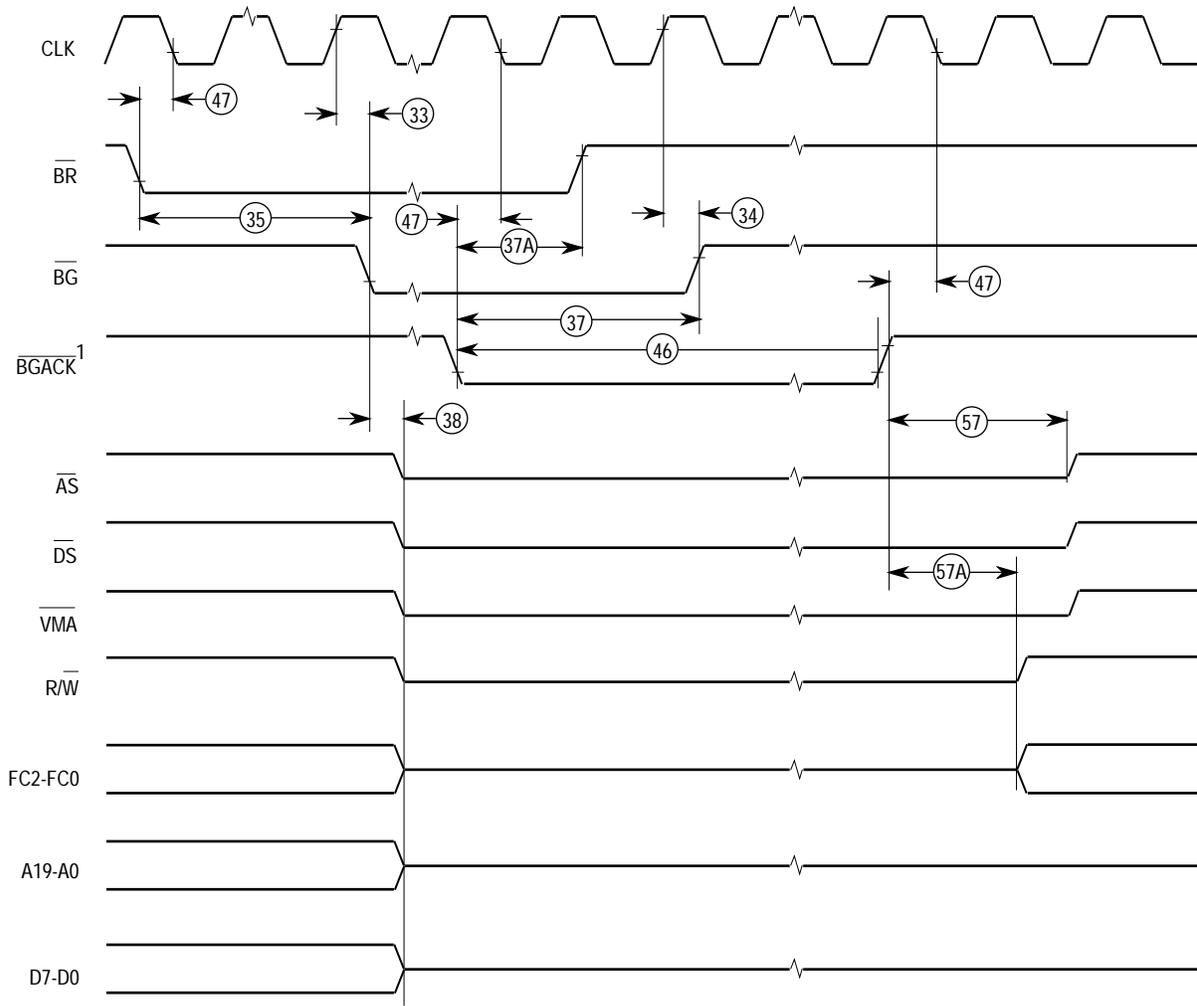
NOTES: Waveform measurements for all inputs and outputs are specified at: logic high 2.0 V, logic low = 0.8 V.
