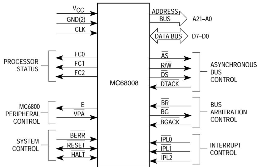
Figure 3-5. Input and Output Signals (MC68008, 52-Pin Version)
