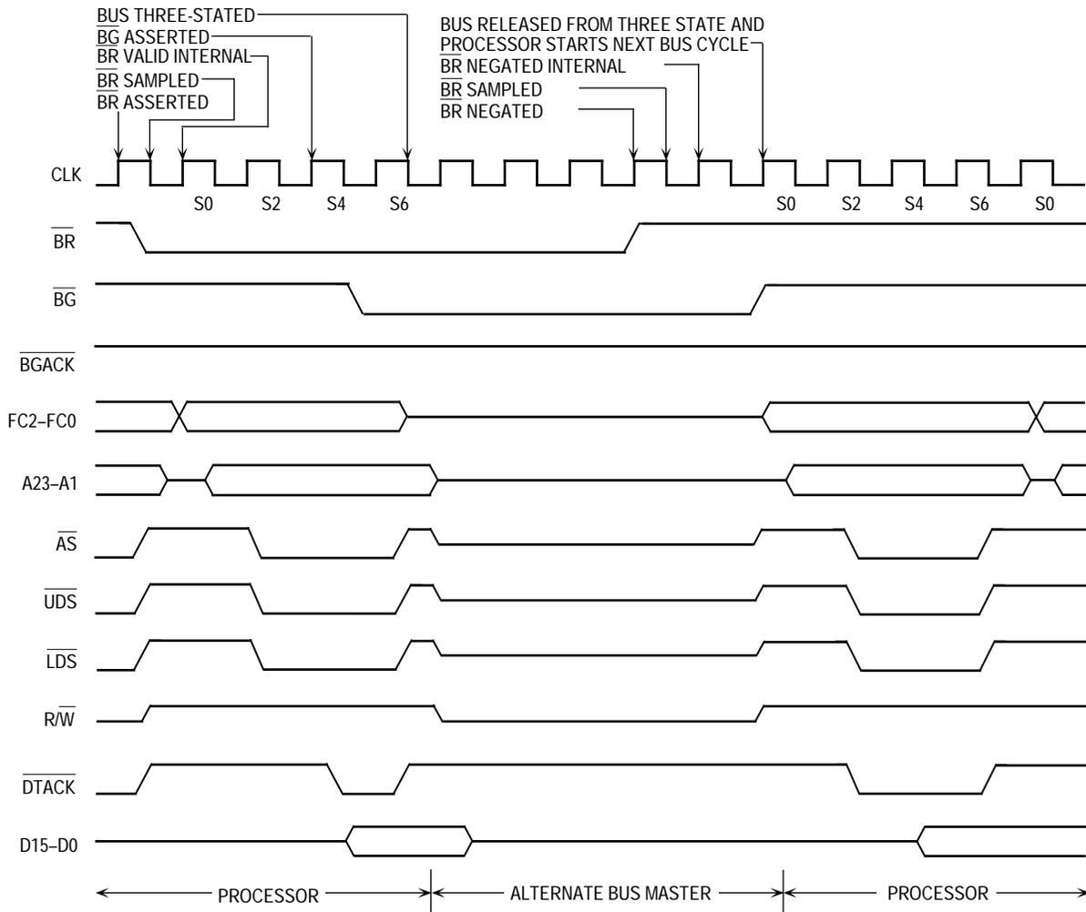
Figure 5-24. 2-Wire Bus Arbitration Timing Diagram—Special Case
