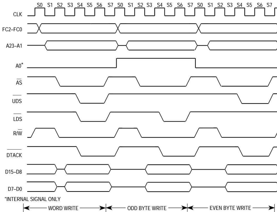
Figure 5-7. Word and Byte Write-Cycle Timing Diagram
