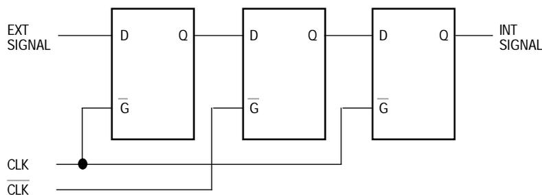
**Figure 5-37. Input Synchronizers**
