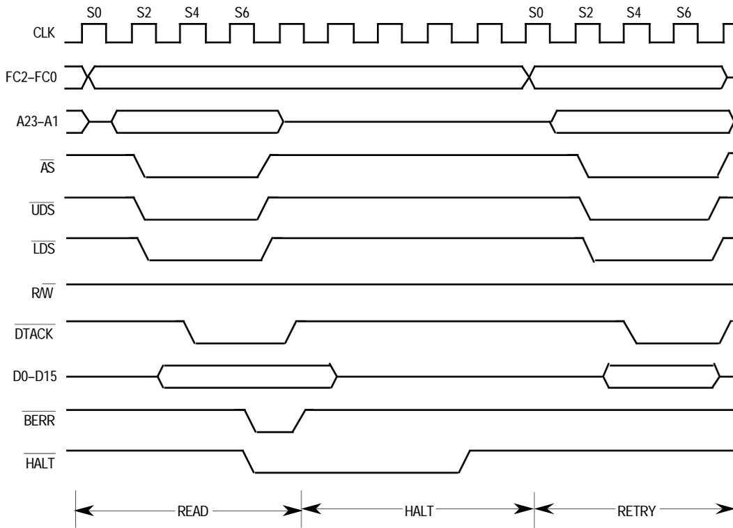
Figure 5-28. Delayed Retry Bus Cycle Timing Diagram
