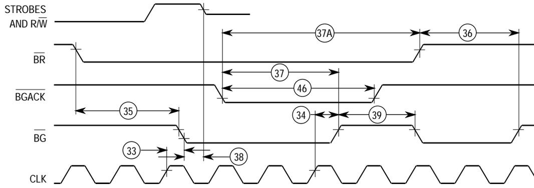
NOTE: Setup time to the clock (#47) for the asynchronous inputs  $\overline{BERR}$ ,  $\overline{BGACK}$ ,  $\overline{BR}$ ,  $\overline{DTACK}$ ,  $\overline{IPL2}$ - $\overline{IPL0}$ , and  $\overline{VPA}$  guarantees their recognition at the next falling edge of the clock.
