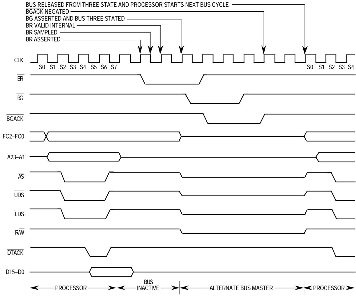
Figure 5-20. 3-Wire Bus Arbitration Timing Diagram—Bus Inactive
