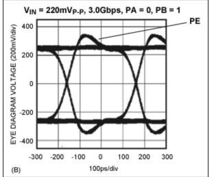
Figure 2B. PE adds amplitude every time that a bit transitions from a 1 to a 0 or a 0 to a 1.
