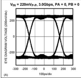
Figure 2A. The eye diagram for the output of the MAX4951BE, which easily meets the =  $400mV_{P-P}$  signal requirement.
