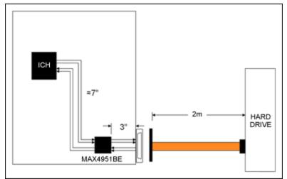
Figure 1. A typical eSATA-to-SATA setup. The host drives several inches of board or cable to the eSATA connector and a 2m eSATA cable to the hard drive.
