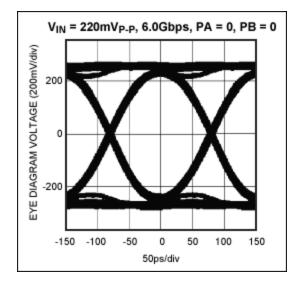
Figure 5. From a 6.0Gbps signal, the MAX4951BE produces an open eye with minimal jitter and is ready for use with the anticipated eSATA specification.
