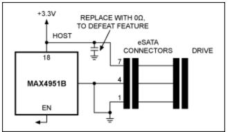
Figure 4. Setup for automated power-down with the MAX4951BE.
