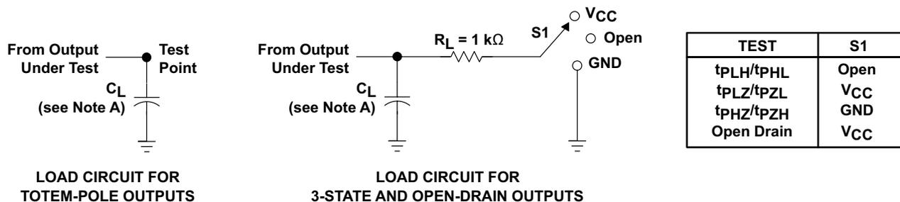
LOAD CIRCUIT FOR TOTEM-POLE OUTPUTS
