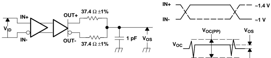
NOTE: All input pulses are supplied by a generator having the following characteristics:  $t_r$  or  $t_f \leq 1$  ns, pulse-repetition rate (PRR) = 0.5 Mpps, pulse width =  $500 \pm 10$  ns;  $R_L = 100 \Omega$ ;  $C_L$  includes instrumentation and fixture capacitance within 0,06 mm of the D.U.T.; the measurement of  $V_{OC(PP)}$  is made on test equipment with a  $-3$  dB bandwidth of at least 300 MHz.
