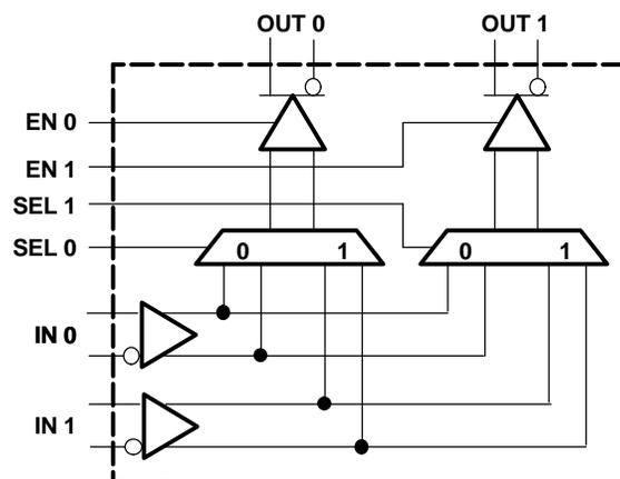
EQUIVALENT INPUT AND OUTPUT SCHEMATIC DIAGRAMS
