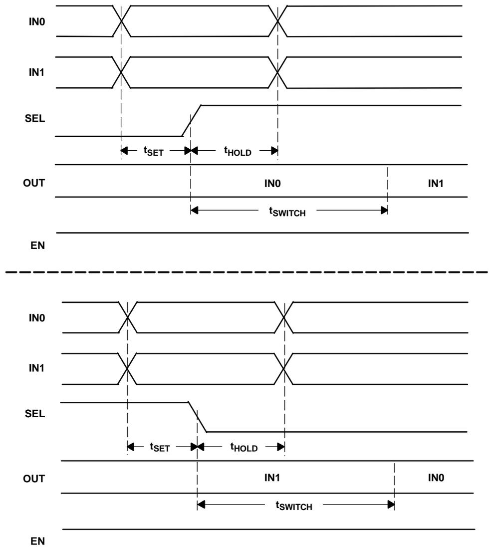
NOTE:  $t_{SET}$  and  $t_{HOLD}$  times specify that data must be in a stable state before and after mux control switches.
