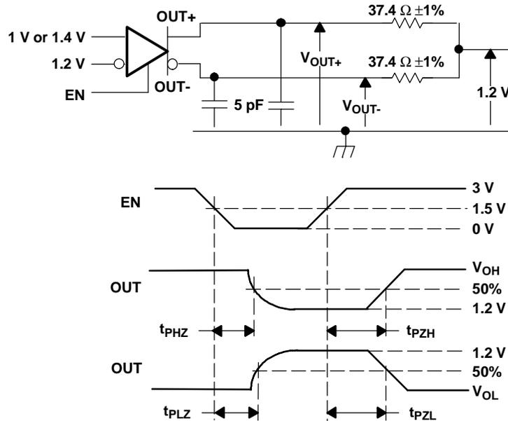
NOTE: All input pulses are supplied by a generator having the following characteristics:  $t_r$  or  $t_f \leq 1$  ns, pulse-repetition rate (PRR) = 0.5 Mpps, pulse width =  $500 \pm 10$  ns.  $C_L$  includes instrumentation and fixture capacitance within 0,06 mm of the D.U.T.
