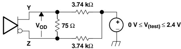
Figure 2. Differential Output Voltage ( $V_{OD}$ ) Test Circuit
