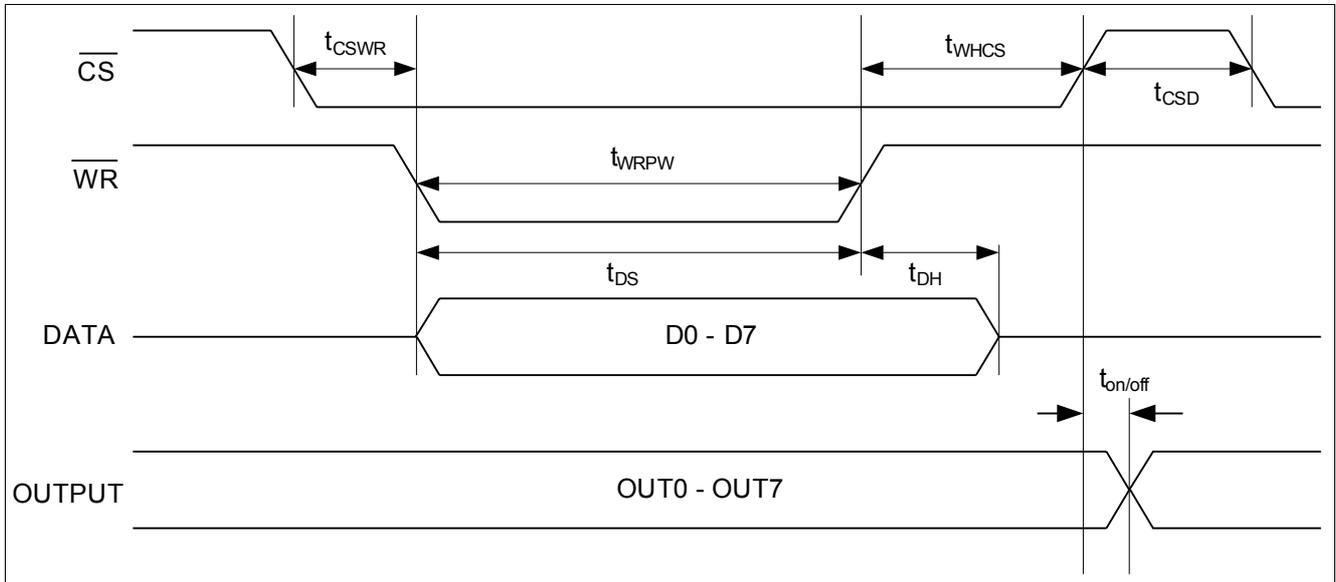
**Figure 10** Parallel input - output timing diagram
