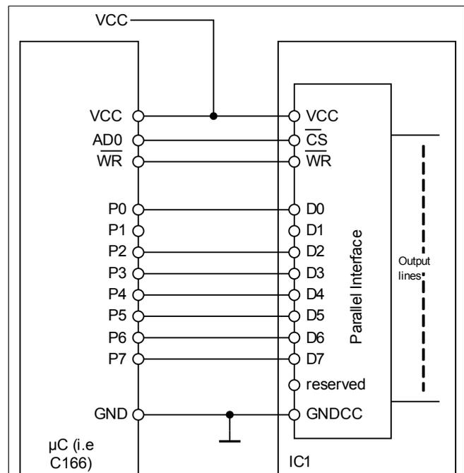
**Figure 8** Parallel bus configuration
