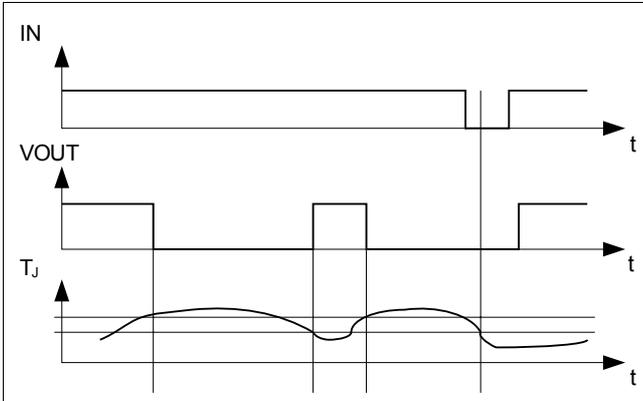
**Figure 5 Overtemperature detection**
