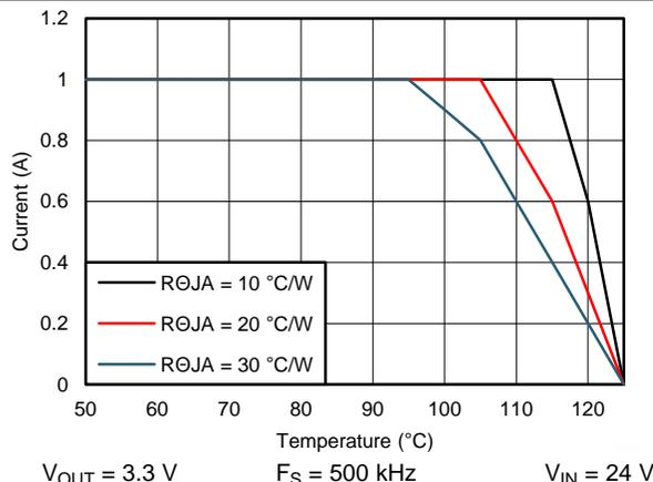
Figure 52. Derating Curve
