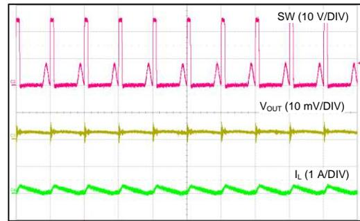
$V_{OUT} = 3.3\text{ V}$        $F_S = 500\text{ kHz}$        $I_{OUT} = 90\text{ mA}$
