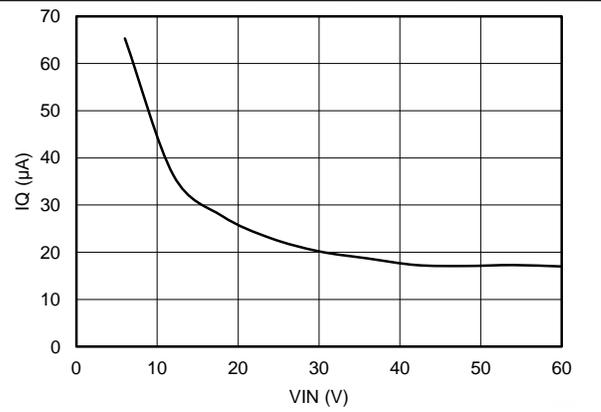
$V_{OUT} = 3.3\text{ V}$        $F_S = 500\text{ kHz}$        $I_{OUT} = 0\text{ A}$
