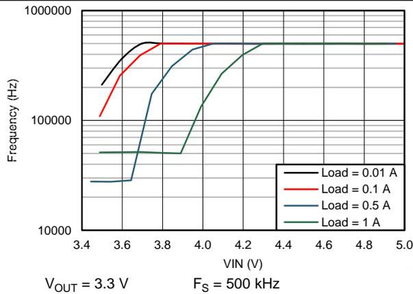
Figure 19. Switching Frequency vs  $V_{IN}$  in Dropout Operation
