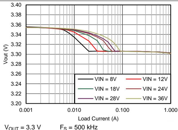
Figure 7.  $V_{OUT}$  Regulation
