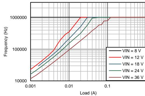
**Figure 34. Switching Frequency Decreases with Lower Load Current in PFM Operation**
