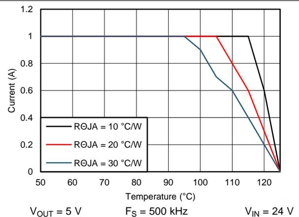
Figure 58. Derating Curve
