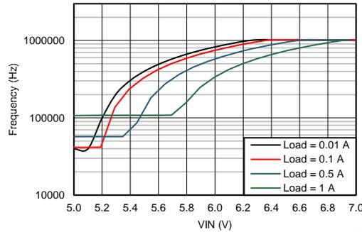
Figure 42. Switching Frequency Decreases in Dropout Operation
