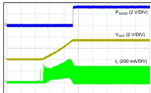
$V_{IN} = 24\text{ V}$        $V_{OUT} = 3.3\text{ V}$        $R_{LOAD} = 33\ \Omega$
