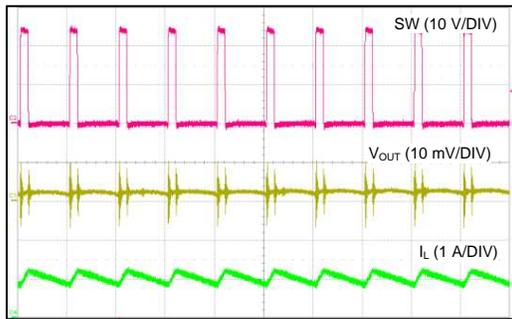
$V_{OUT} = 3.3\text{ V}$        $F_S = 500\text{ kHz}$        $I_{OUT} = 1\text{ A}$
