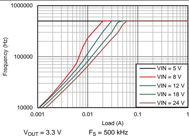
Figure 87. Switching Frequency vs  $I_{OUT}$  in PFM Operation
