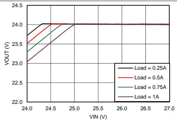
$V_{OUT} = 24\text{ V}$   $F_S = 500\text{ kHz}$
