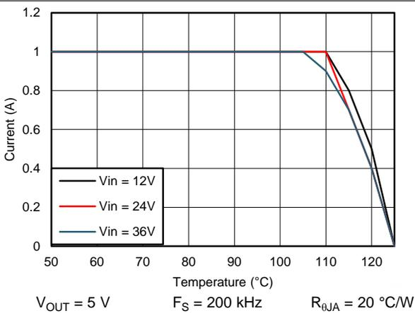
Figure 85. Derating Curve with  $R_{\theta JA} = 20^\circ\text{C/W}$
