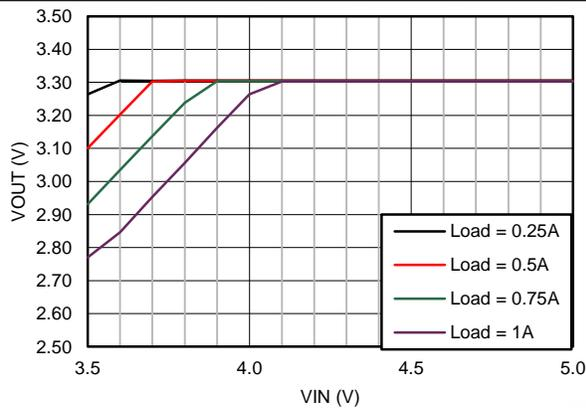
$V_{OUT} = 3.3\text{ V}$   $F_S = 500\text{ kHz}$
