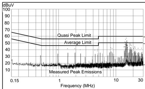
Measured on LM46001PWPEVM with default BOM. EVM input filter:  $L_{in} = 1\text{ }\mu\text{H}$ ,  $C_d = 47\text{ }\mu\text{F}$ ,  $C_{IN4} = 68\text{ }\mu\text{F}$
