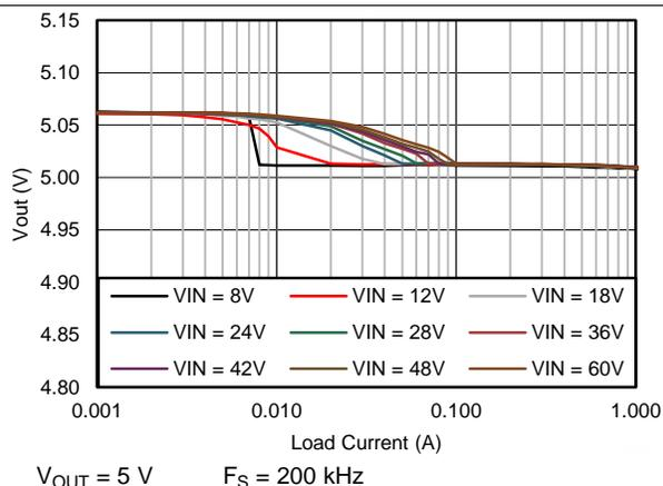
Figure 9.  $V_{OUT}$  Regulation
