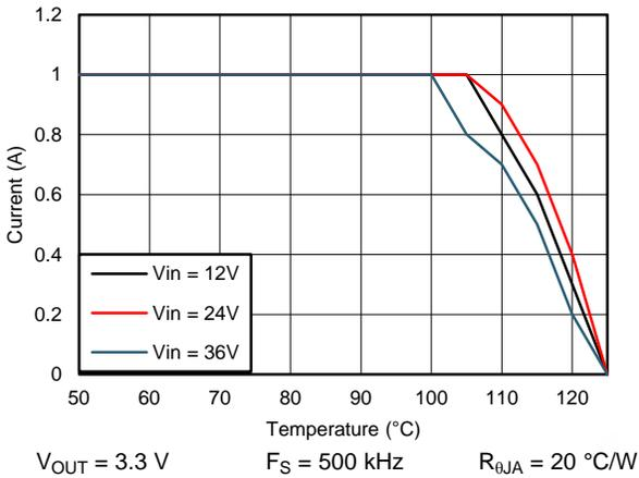
Figure 83. Derating Curve with  $R_{\theta JA} = 20^\circ\text{C/W}$
