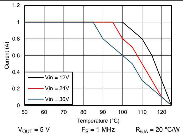
Figure 86. Derating Curve with  $R_{\theta JA} = 20^\circ\text{C/W}$
