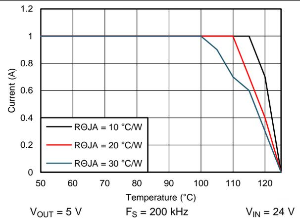
Figure 64. Derating Curve
