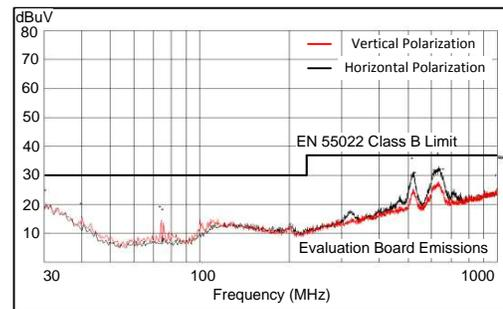
Measured on the LM46001PWPEVM with  $L = 27\text{ }\mu\text{H}$ ,  $C_{OUT} = 66\text{ }\mu\text{F}$ ,  $C_{FF} = 33\text{ pF}$ . No input filter used.
