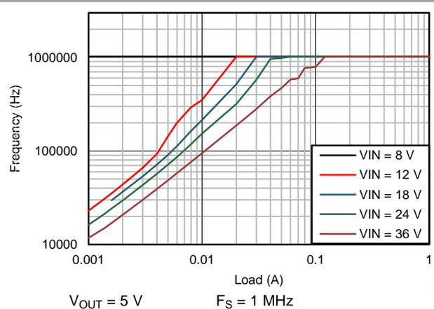
Figure 88. Switching Frequency vs  $I_{OUT}$  in PFM Operation
