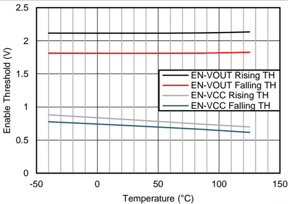
Figure 27. Enable Threshold vs Junction Temperature
