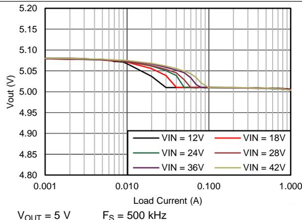
Figure 8.  $V_{OUT}$  Regulation
