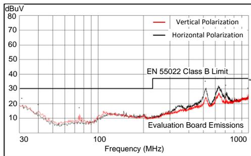
Measured on the LM46001PWPEVM with default BOM. No input filter used.
