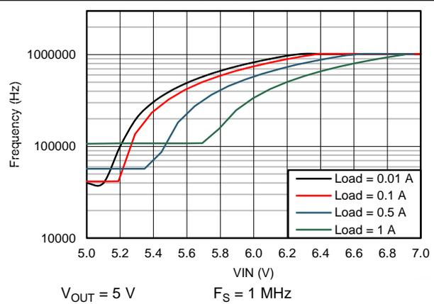
Figure 20. Switching Frequency vs  $V_{IN}$  in Dropout Operation
