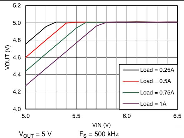
Figure 56. Dropout Curve
