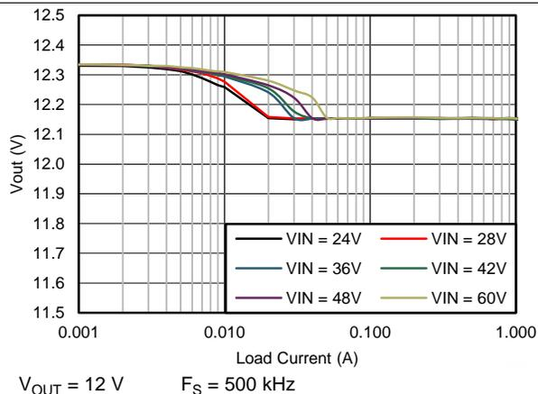
Figure 11.  $V_{OUT}$  Regulation
