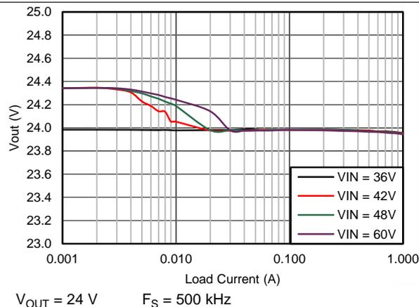
Figure 12.  $V_{OUT}$  Regulation
