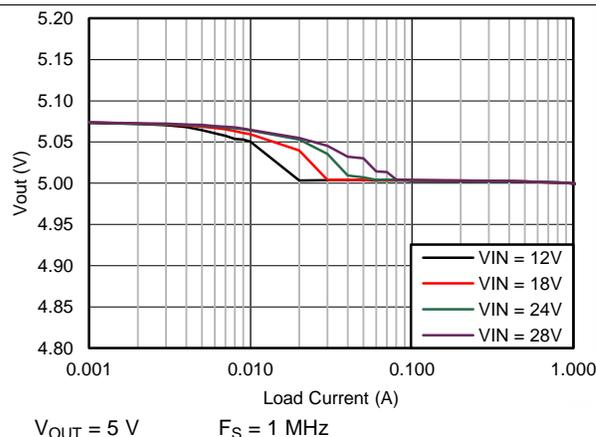
Figure 10.  $V_{OUT}$  Regulation
