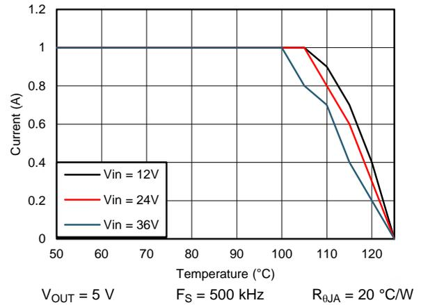
Figure 84. Derating Curve with  $R_{\theta JA} = 20^\circ\text{C/W}$
