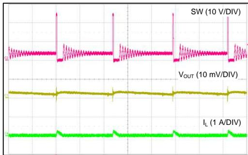
$V_{OUT} = 3.3\text{ V}$        $F_S = 500\text{ kHz}$        $I_{OUT} = 10\text{ mA}$
