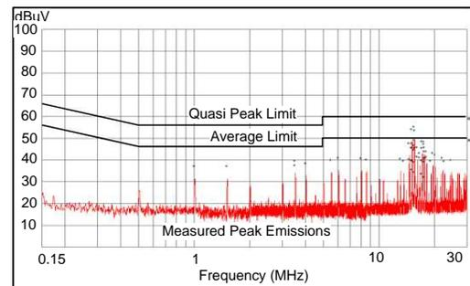
Measured on LM46001PWPEVM with  $L = 27\text{ }\mu\text{H}$ ,  $C_{OUT} = 66\text{ }\mu\text{F}$ ,  $C_{FF} = 33\text{ pF}$ . EVM input filter  $L_{in} = 1\text{ }\mu\text{H}$ ,  $C_d = 47\text{ }\mu\text{F}$ ,  $C_{IN4} = 68\text{ }\mu\text{F}$
