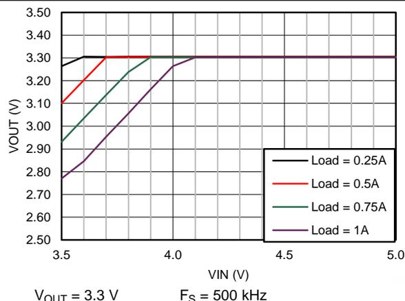
Figure 50. Dropout Curve
