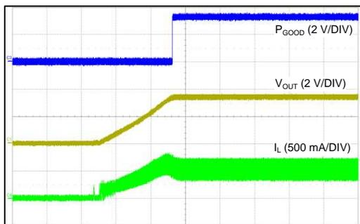
$V_{IN} = 24\text{ V}$        $V_{OUT} = 3.3\text{ V}$        $R_{LOAD} = 6.6\ \Omega$
