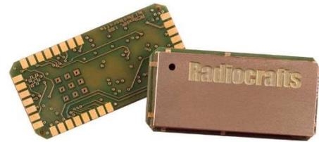
The module contains a complete IEEE802.15.4g/e compliant stack which is accessed through an API via UART. Through the free middleware, *RIIoT Net Controller*, the interface to the RIIoT network is accessible through a local socket interface. This enables easy development of customer applications that can include fog computing or cloud connection through MQTT or RESTful HTTP.
