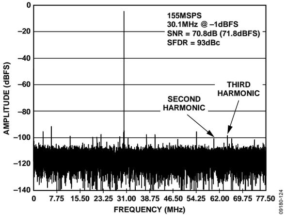
Figure 24. AD9644-155 Single-Tone FFT with  $f_{IN} = 30.1$  MHz
