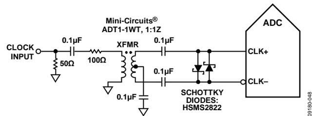
Figure 54. Transformer-Coupled Differential Clock (Up to 200 MHz)
