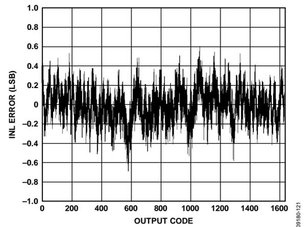
Figure 21. AD9644-80 INL with  $f_{IN} = 30.3$  MHz
