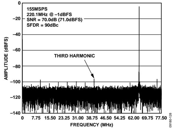
Figure 28. AD9644-155 Single-Tone FFT with  $f_{IN} = 220.1$  MHz
