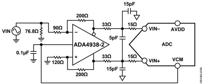
Figure 49. Differential Input Configuration Using the ADA4938-2
