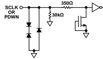
Figure 45. Equivalent SCLK or PDWN Input Circuit
