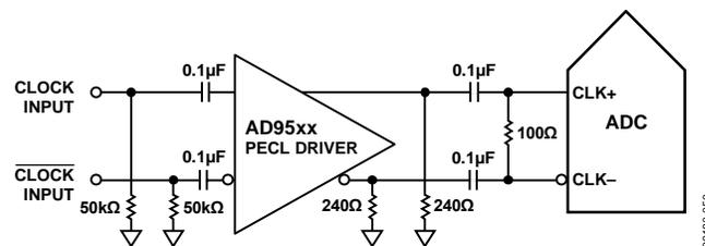
Figure 56. Differential PECL Sample Clock (Up to 640 MHz)
