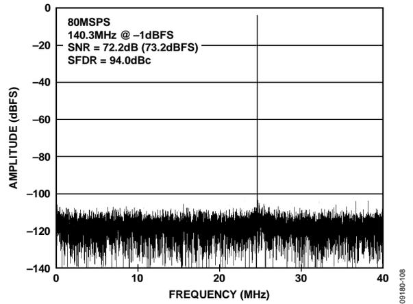
Figure 8. AD9644-80 Single-Tone FFT with  $f_{IN} = 140.1$  MHz
