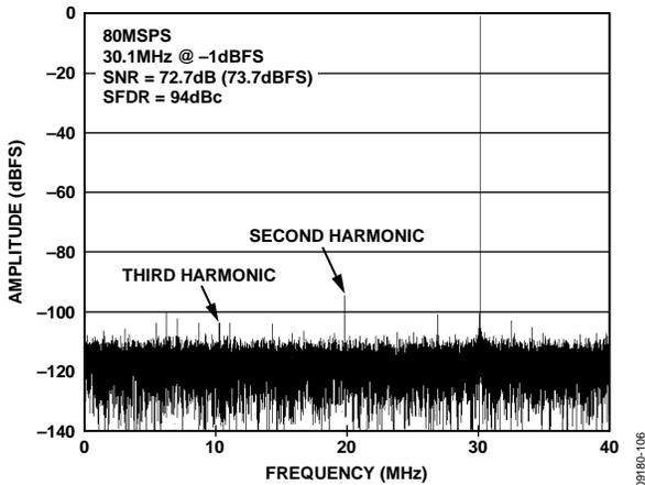
Figure 6. AD9644-80 Single-Tone FFT with  $f_{IN} = 30.1$  MHz
