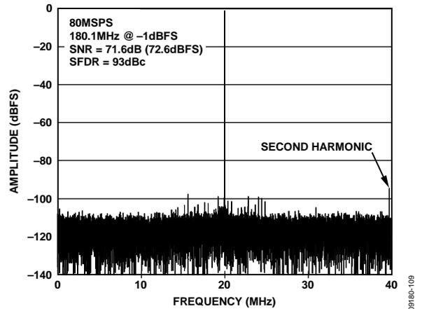
Figure 9. AD9644-80 Single-Tone FFT with  $f_{IN} = 180.1$  MHz
