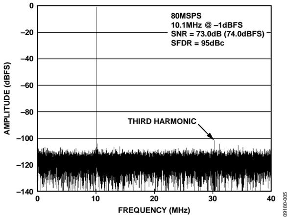
Figure 5. AD9644-80 Single-Tone FFT with  $f_{IN} = 10.1$  MHz
