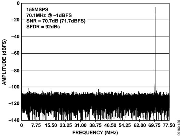
Figure 25. AD9644-155 Single-Tone FFT with  $f_{IN} = 70.1$  MHz
