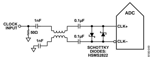
Figure 55. Balun-Coupled Differential Clock (Up to 640 MHz)
