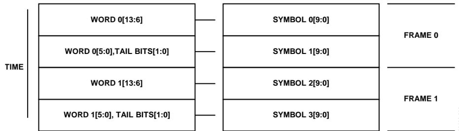
Figure 64. AD9644 14-Bit Data Transmission with Tail Bits
