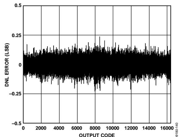
Figure 40. AD9644-155 DNL with  $f_{IN} = 30.3$  MHz
