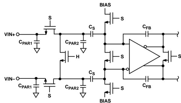
Figure 48. Switched-Capacitor Input
