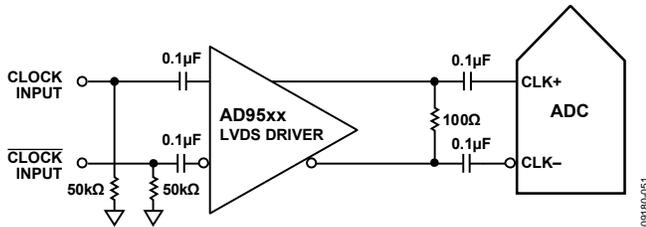
Figure 57. Differential LVDS Sample Clock (Up to 640 MHz)
