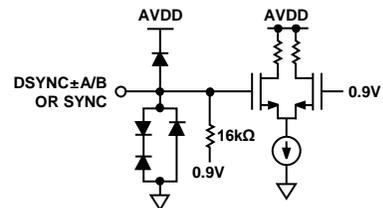
Figure 47. Equivalent SYNC and DSYNC Input Circuit
