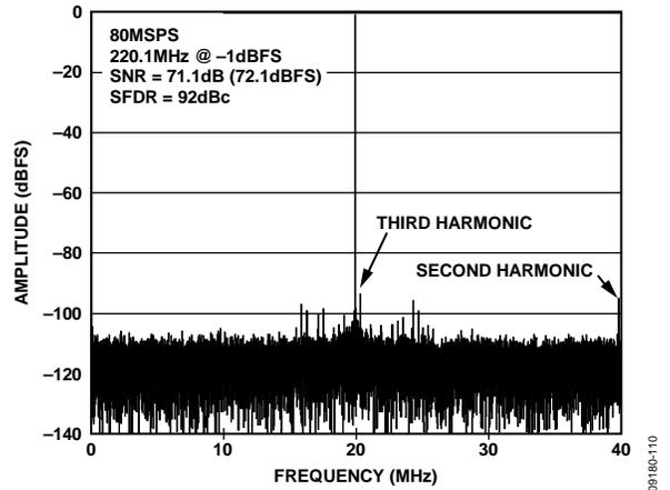
Figure 10. AD9644-80 Single-Tone FFT with  $f_{IN} = 220.1$  MHz
