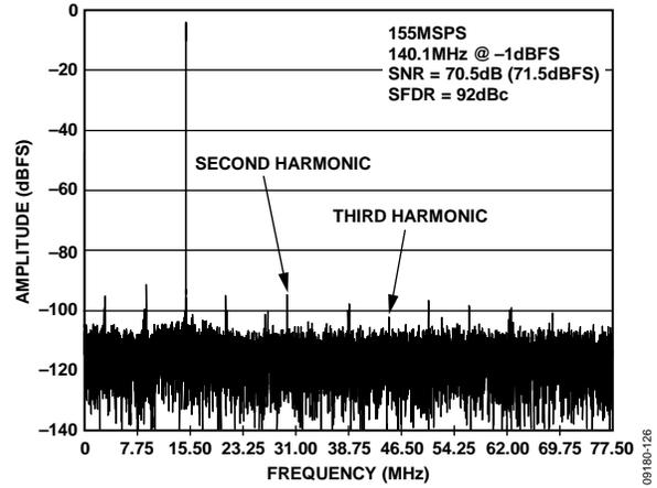
Figure 26. AD9644-155 Single-Tone FFT with  $f_{IN} = 140.1$  MHz
