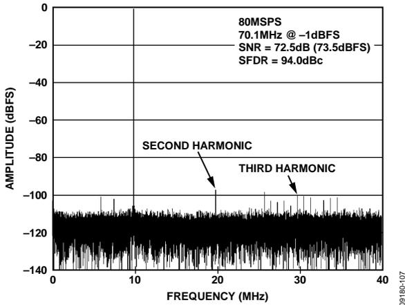
Figure 7. AD9644-80 Single-Tone FFT with  $f_{IN} = 70.1$  MHz
