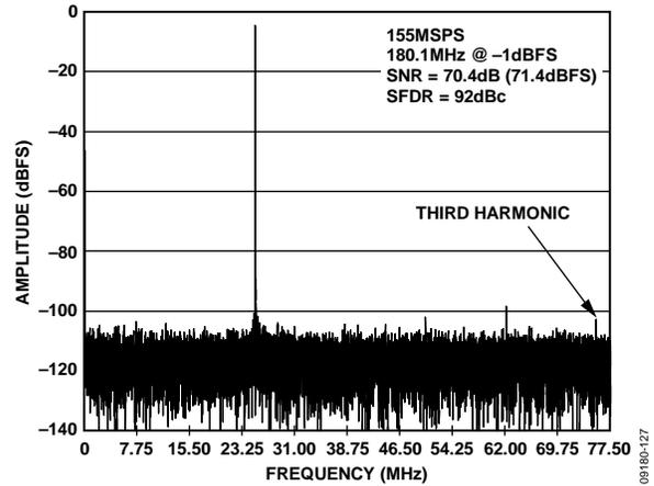
Figure 27. AD9644-155 Single-Tone FFT with  $f_{IN} = 180.1$  MHz
