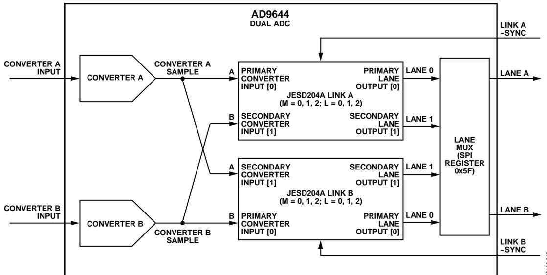
Figure 62. AD9644 Transmit Link Simplified Block Diagram
