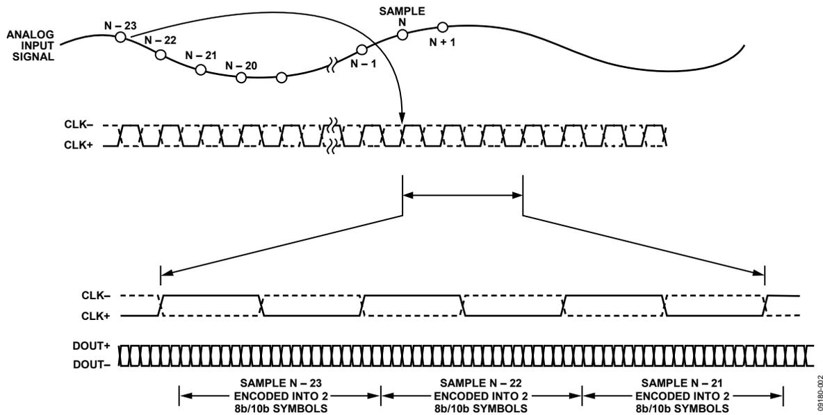
Figure 2. Data Output Timing
