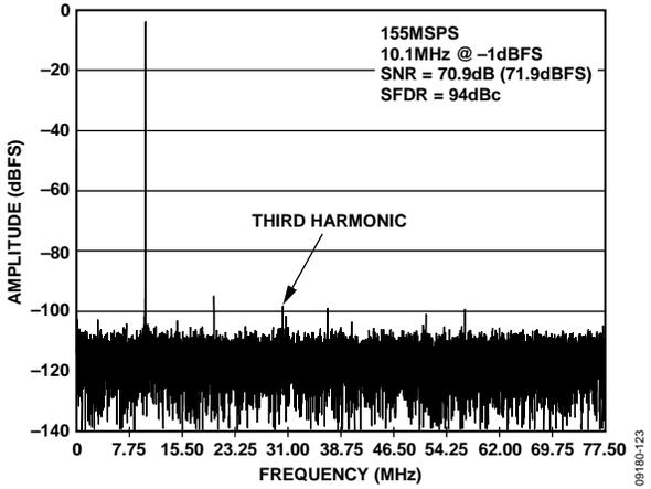
Figure 23. AD9644-155 Single-Tone FFT with  $f_{IN} = 10.1$  MHz
