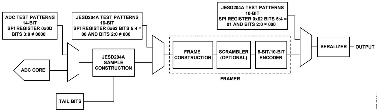
Figure 70. Block Diagram Showing Digital Test Modes
