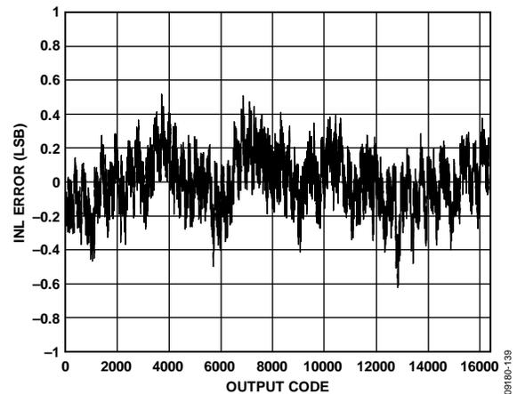
Figure 39. AD9644-155 INL with  $f_{IN} = 30.3$  MHz
