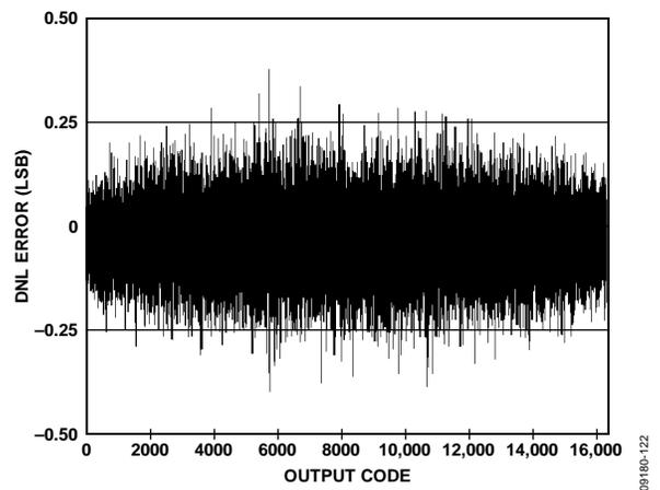
Figure 22. AD9644-80 DNL with  $f_{IN} = 30.3$  MHz
