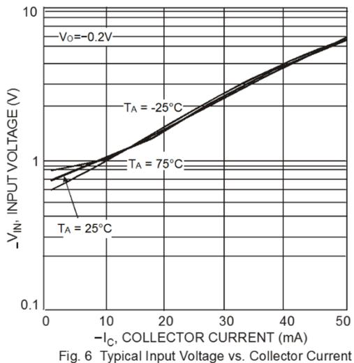
**Typical Curves – DCX123JU NPN Section (@  $T_A = +25^\circ\text{C}$ , unless otherwise specified.)**
