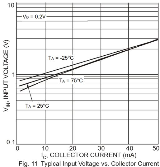
**Typical Curves – DCX143EU PNP Section** (@  $T_A = +25^\circ\text{C}$ , unless otherwise specified.)
