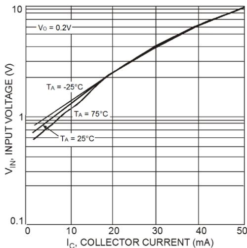
Fig. 33 Typical Input Voltage vs. Collector Current
