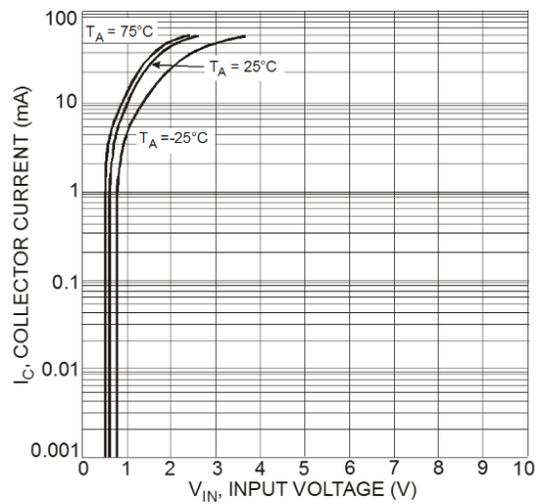
Fig. 32 Typical Collector Current vs. Input Voltage
