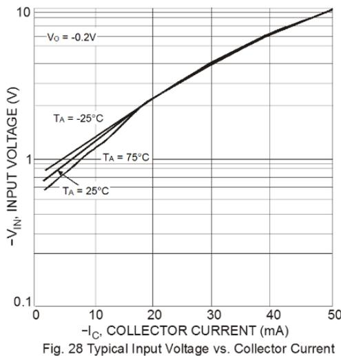
**Typical Curves – DCX114TU NPN Section** (@  $T_A = +25^\circ\text{C}$ , unless otherwise specified.)
