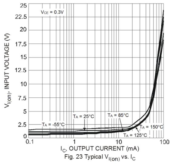
**Typical Curves – DCX114TU PNP Section (@  $T_A = +25^\circ\text{C}$ , unless otherwise specified.)**
