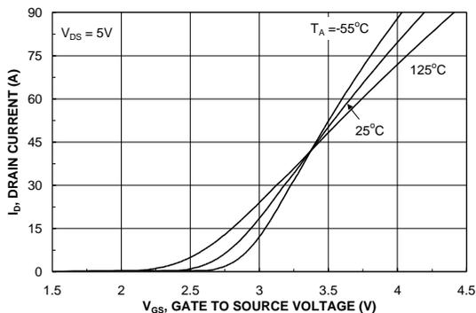
**Figure 5. Transfer Characteristics**
