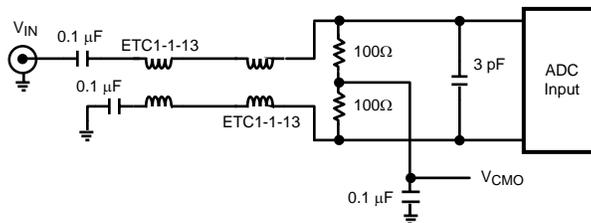
**Figure 22. High Input Frequency Transformer Drive Circuit**
