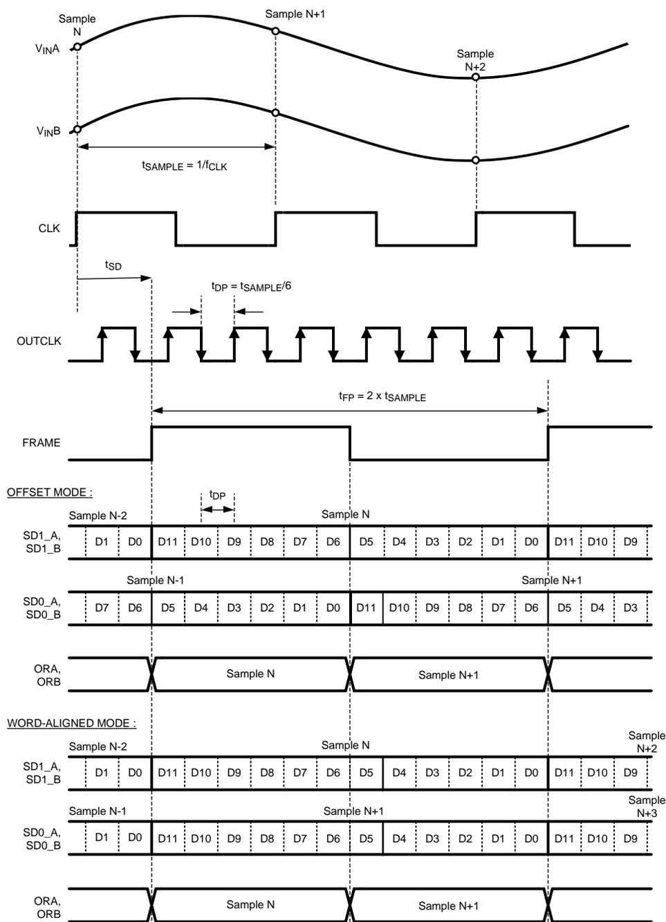
Figure 5. Serial Output Data Format in Dual-Lane Mode
