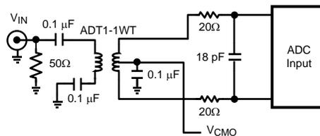
**Figure 21. Low Input Frequency Transformer Drive Circuit**
