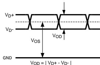
**LVDS Differential Output Voltage ( $V_{OD}$ )** is the absolute value of the difference between the differential output pair voltages ( $V_{D+}$  and  $V_{D-}$ ), each measured with respect to ground.
