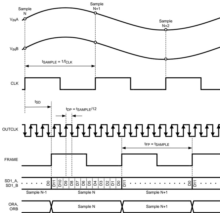
Figure 4. Serial Output Data Format in Single-Lane Mode
