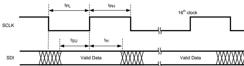
Figure 26. Write Timing
