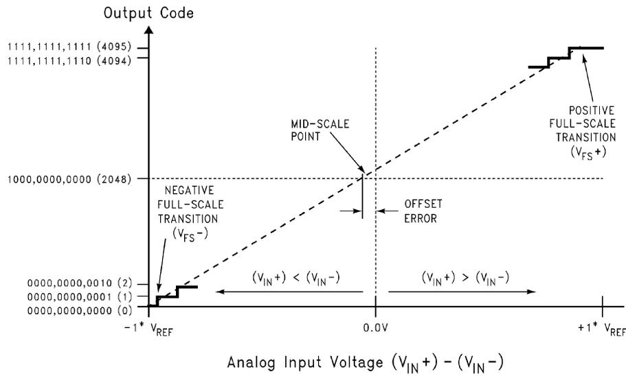
Figure 6. Transfer Characteristic
