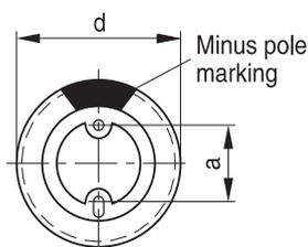
The series B41898 has no sleeve nor minus pole marking, the positive pole is marked on the aluminum case side instead.
