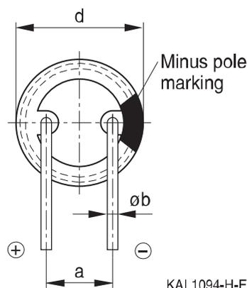
The series B41898 has no sleeve nor minus pole marking, the positive pole is marked on the aluminum case side instead.
