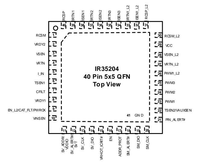
Figure 1: IR35204 Pin Diagram
