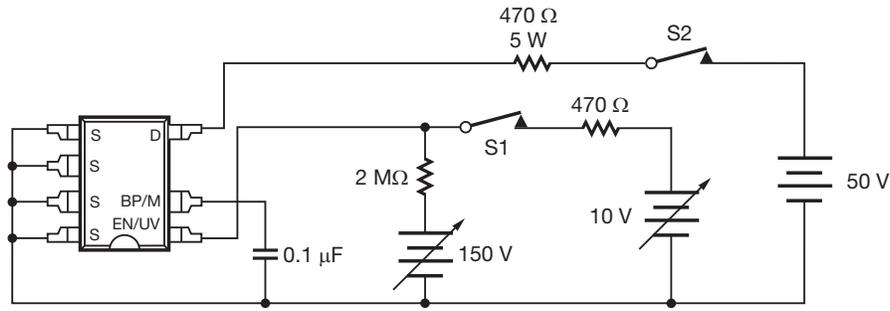
**NOTE:** This test circuit is not applicable for current limit or output characteristic measurements.
