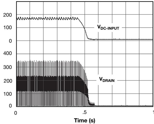
Figure 12. Normal Power Down Timing (without UV).
