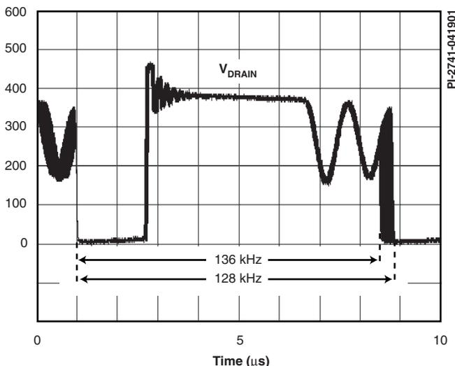
Figure 4. Frequency Jitter.
