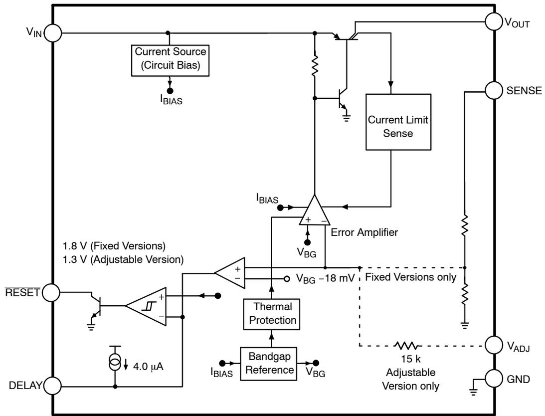
Figure 2. Block Diagram
