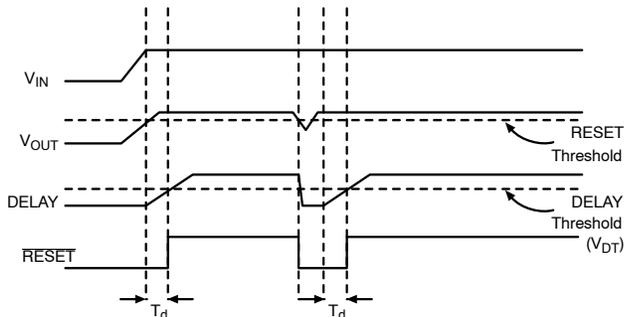
Figure 13. Reset and Delay Circuit Wave Forms
