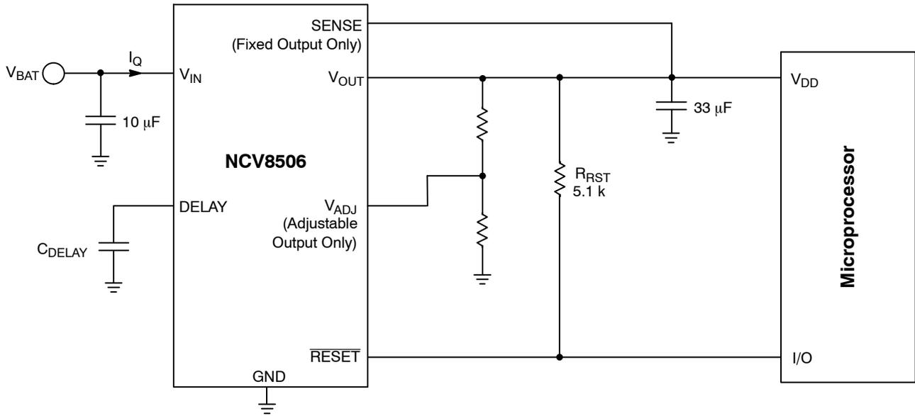
Figure 1. Application Diagram
