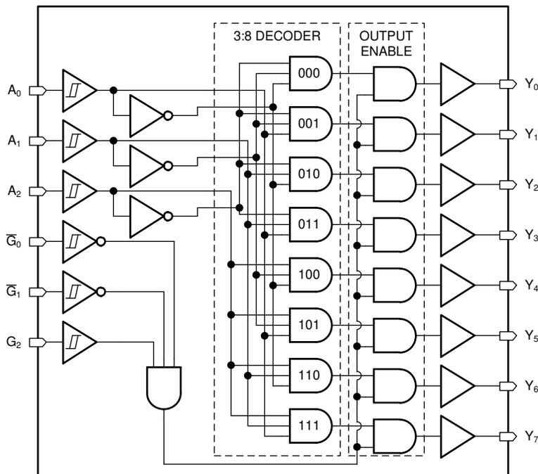
Figure 8-1. Logic Diagram (Positive Logic) for SN74HCS238
