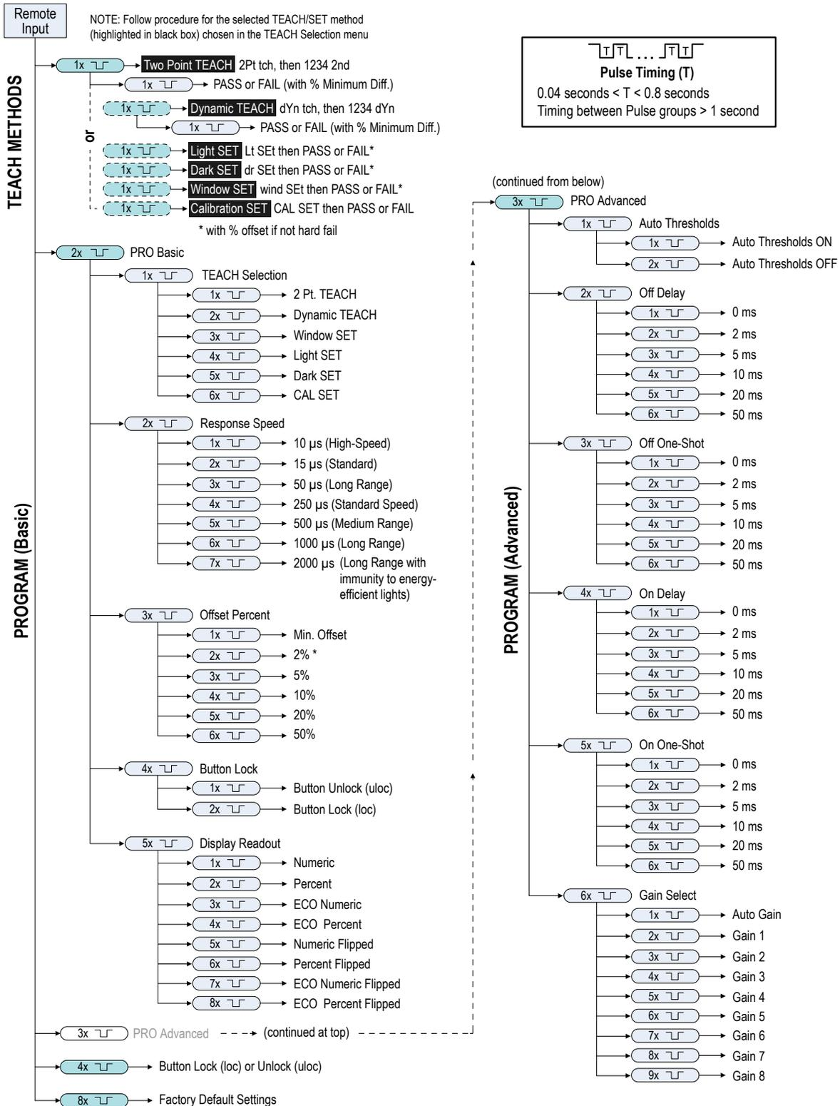
\* In Super High-Speed and High-Speed Responses, 2% offset is forced to Min. Offset
