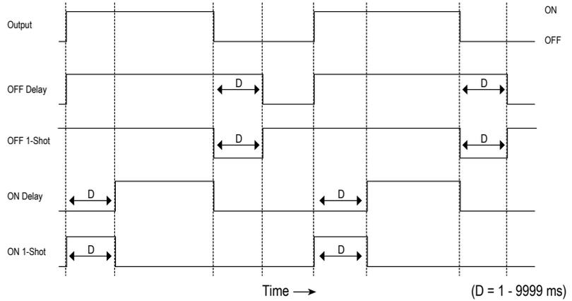
Figure 3. DF-G2 Delays/Timers
