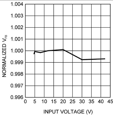
Figure 9. Normalized Feedback Voltage vs Input Voltage
