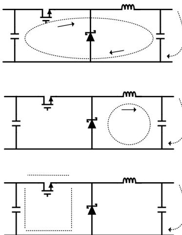
Figure 22. Current Flow in a Buck Application
