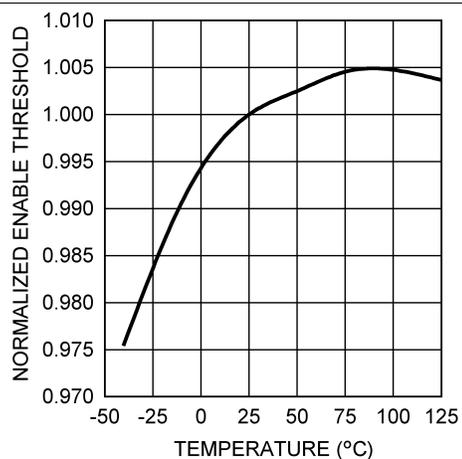
Figure 6. Normalized Enable Threshold Voltage vs Temperature
