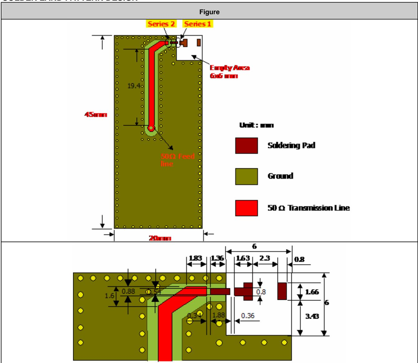
Antenna on Test Board ( Thickness 1.2mm)
