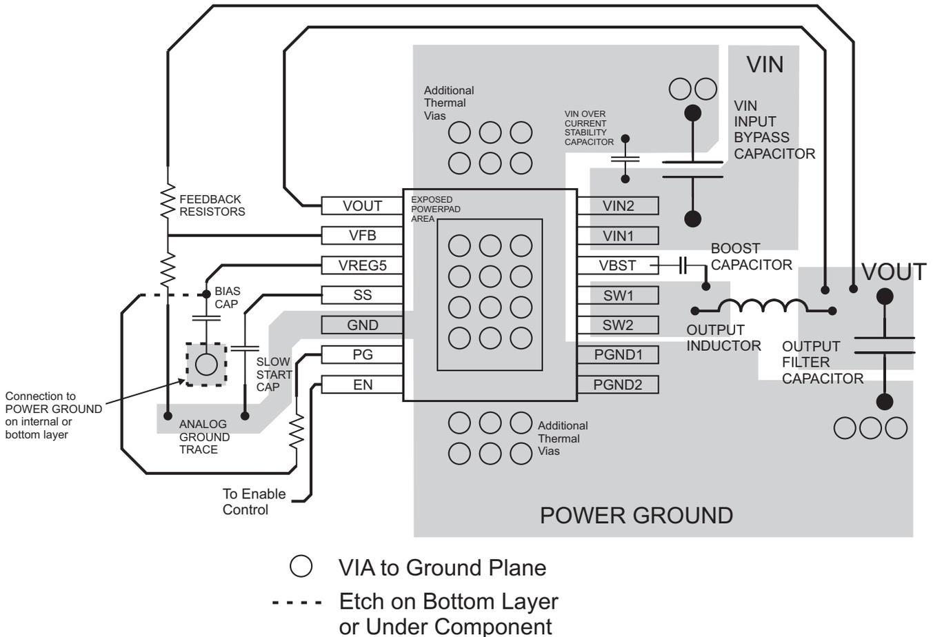
**Figure 17. PCB Layout**
