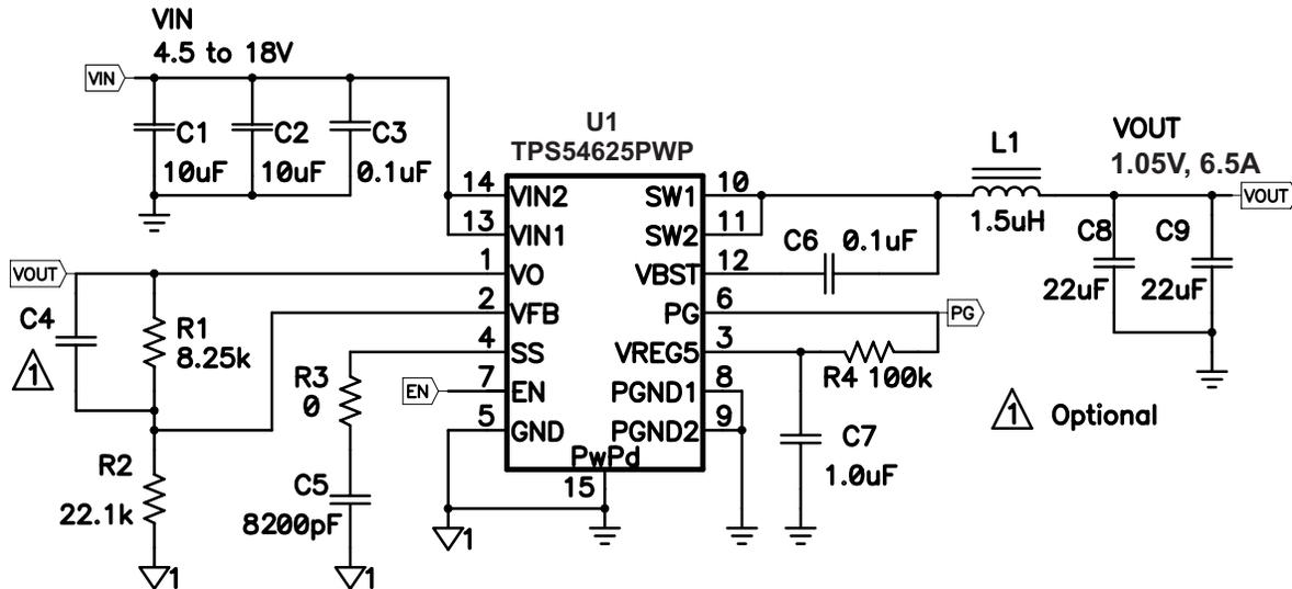
Figure 15. Schematic
