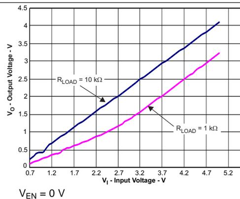
Figure 12. Output Voltage versus Input Voltage, Device Disabled (TPS61220)
