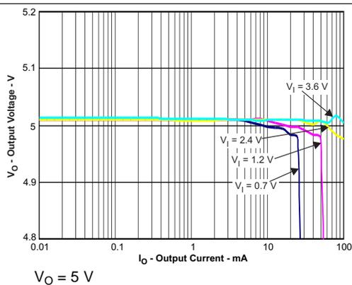
Figure 11. Output Voltage versus Output Current and Input Voltage (TPS61222)
