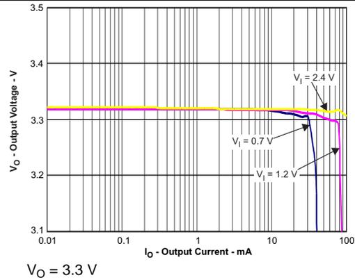
Figure 10. Output Voltage versus Output Current and Input Voltage (TPS61221)
