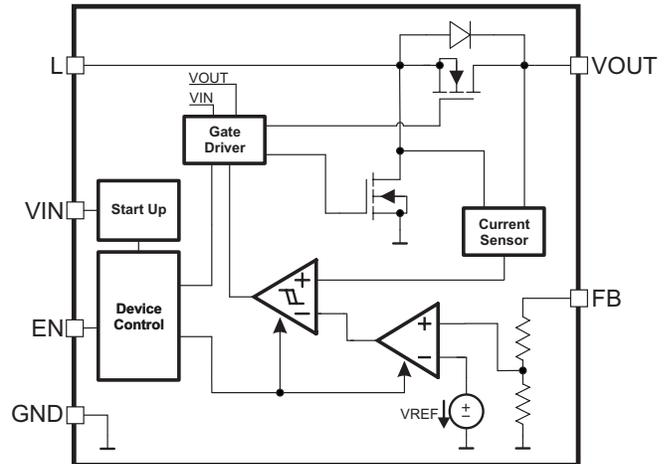
Figure 24. Functional Block Diagram (Fixed Output Voltage Version)
