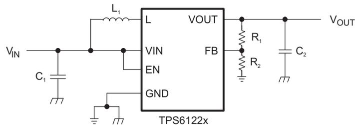
Figure 28. Application Circuit For Adjustable Output Voltage Option
