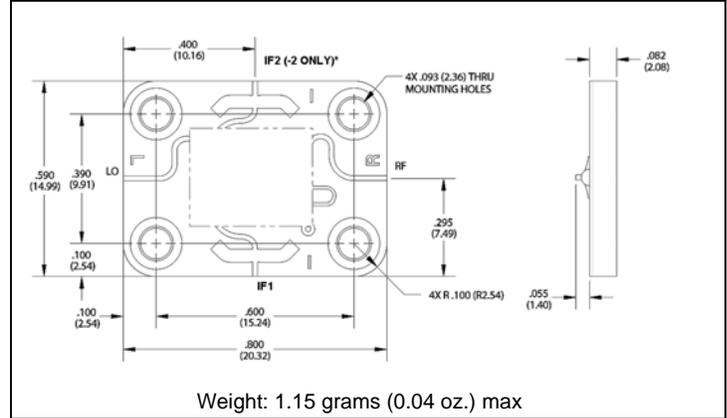
\*For the base model, only IF1 port is connected.
