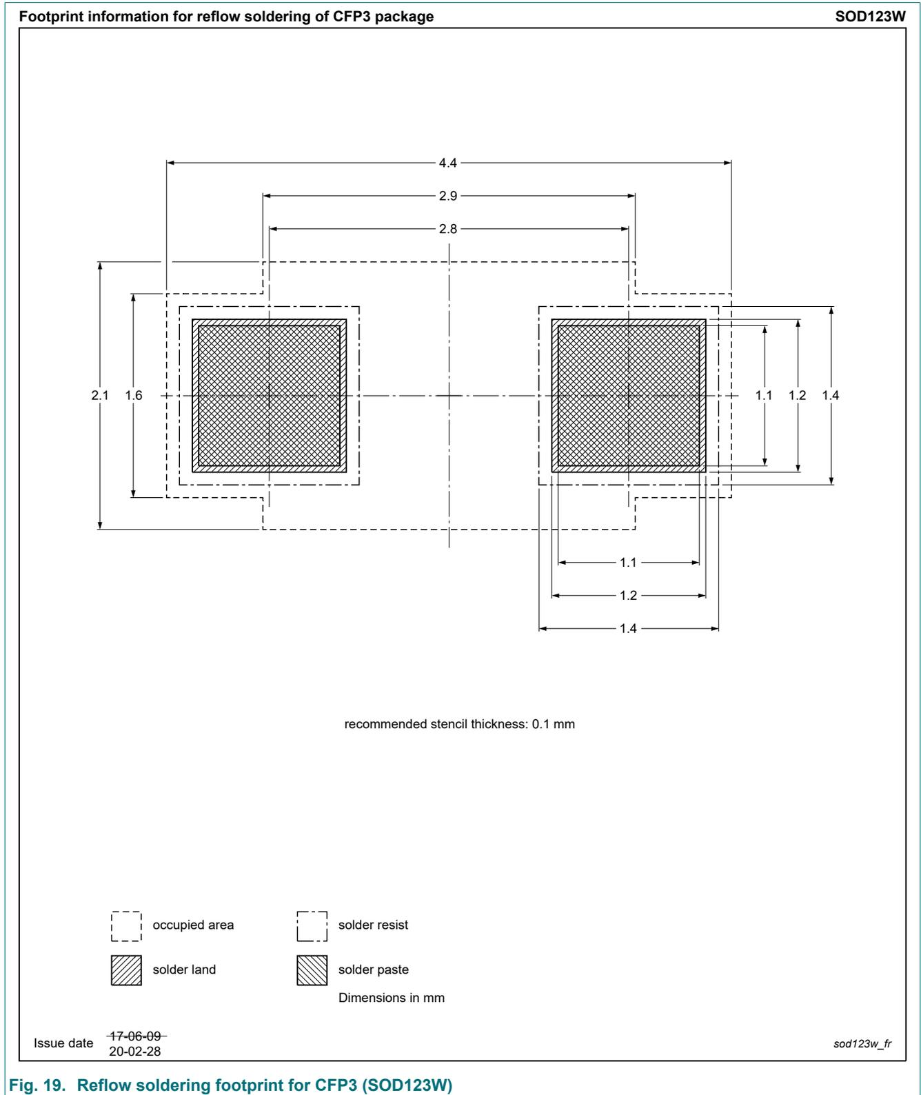
Fig. 19. Reflow soldering footprint for CFP3 (SOD123W)
