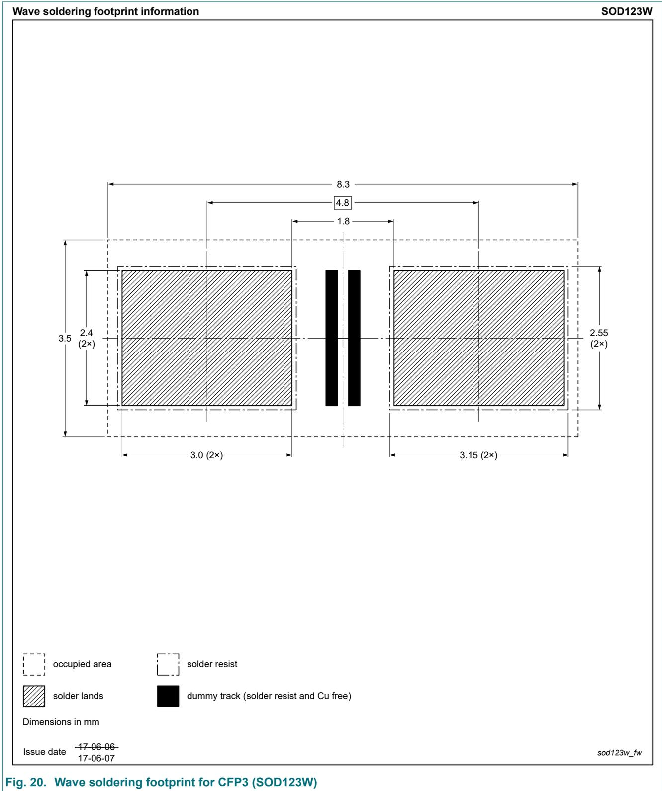
**Fig. 20. Wave soldering footprint for CFP3 (SOD123W)**
