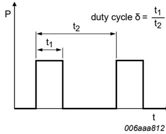
Fig. 17. Duty cycle definition
