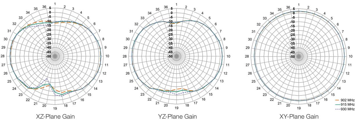
Figure 9. Radiation Patterns for ANT-915-IPW1-RPS, Edge Bent
