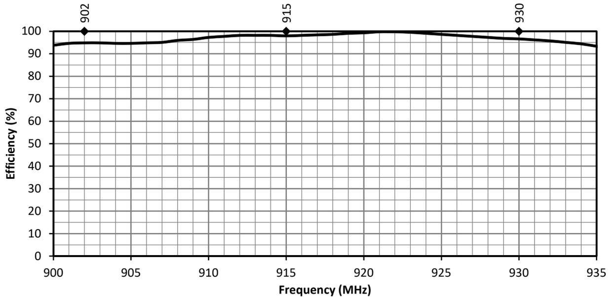
Figure 8. ANT-915-IPW1-RPS Antenna Radiation Efficiency, Edge Bent
