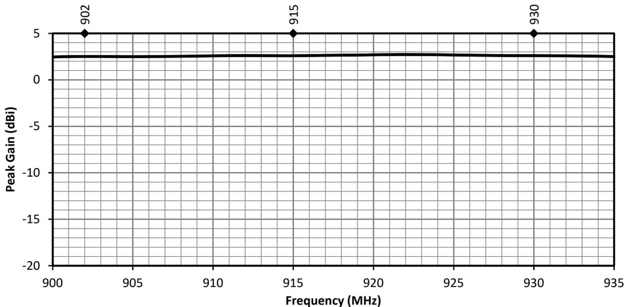
Figure 6. ANT-915-IPW1-RPS Antenna Peak Gain, Edge Bent
