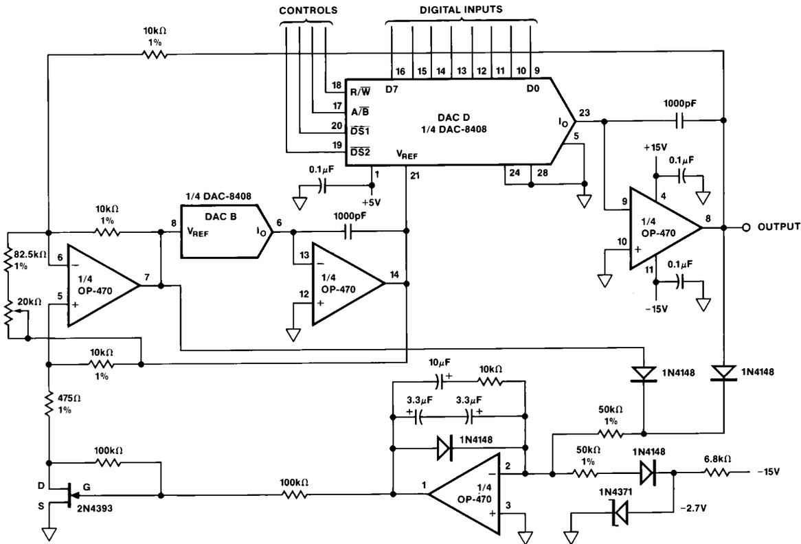
Figure 11. A Digitally Programmable, Low-Distortion Sinewave Oscillator
