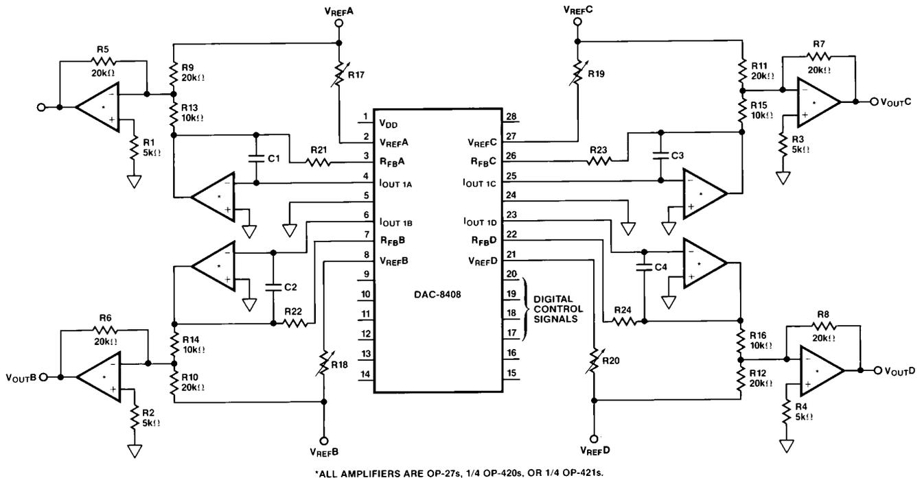
Figure 7. Quad DAC Bipolar Operation (4-Quadrant Multiplication)
