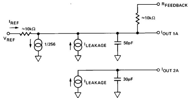
Figure 3. Equivalent DAC Circuit (All Digital Inputs HIGH)
