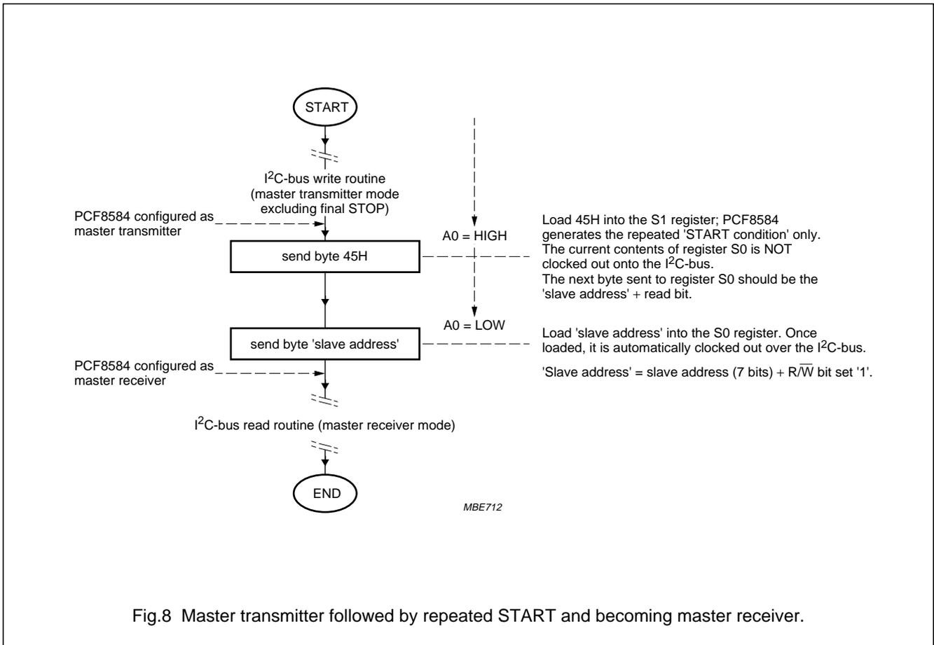
Fig.8 Master transmitter followed by repeated START and becoming master receiver.
