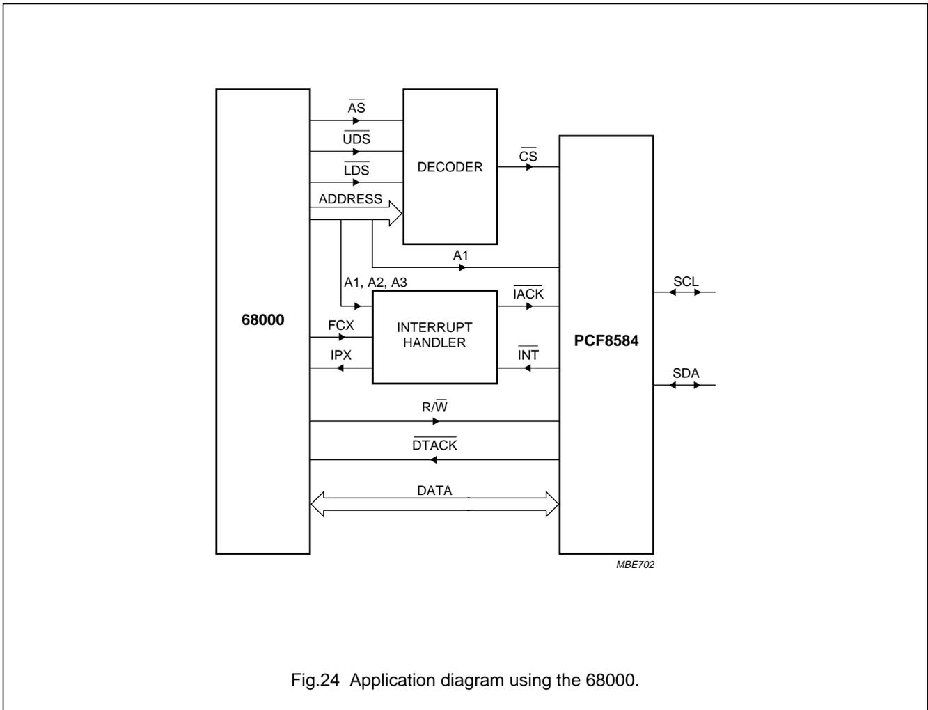
Fig.24 Application diagram using the 68000.
