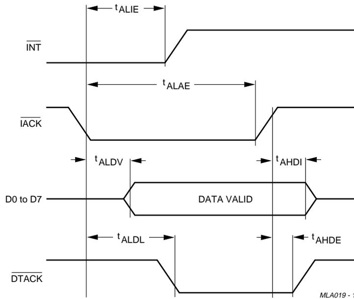
Fig.20 Interrupt timing (68000 mode).
