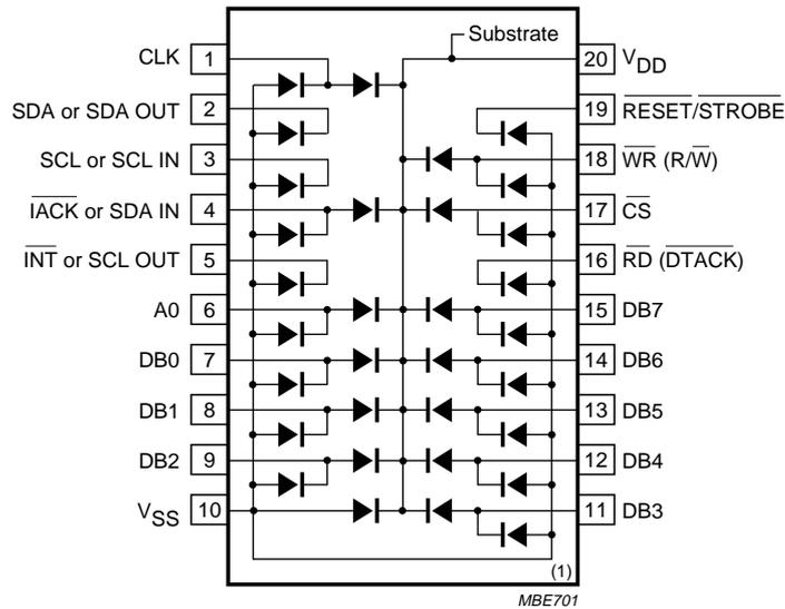
Maximum forward current: 5 mA; maximum reverse voltage: 5 V.
