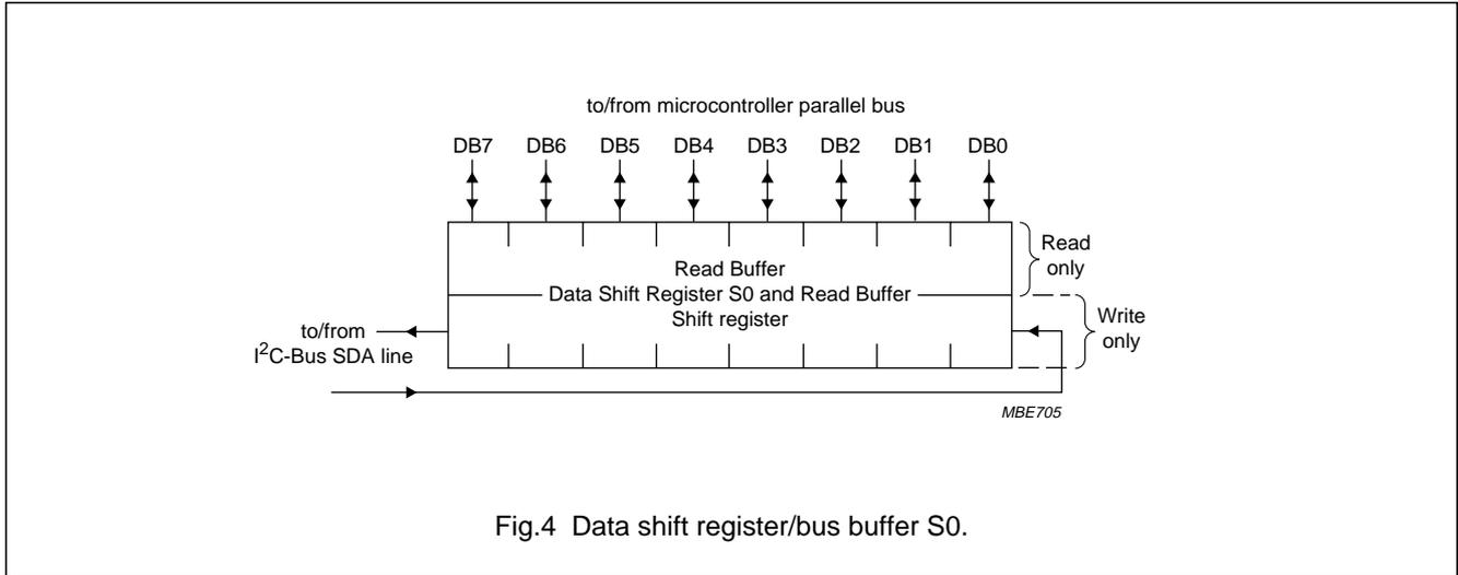
In receiver mode the data from the shift register is copied to the read buffer during the acknowledge phase. Further reception of data is inhibited (SCL held LOW) until the S0 read buffer is read (see Section 6.8.1.1).
