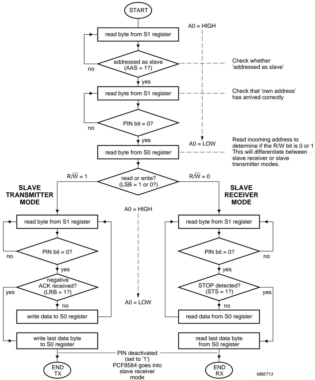
Fig.9 Slave receiver/slave transmitter modes.
