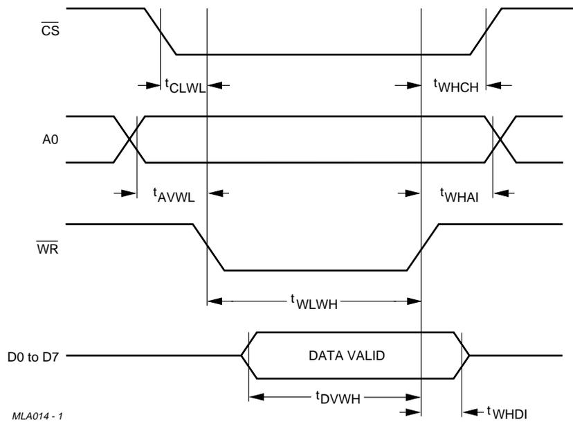
Fig.15 Bus timing (80XX mode); write cycle.
