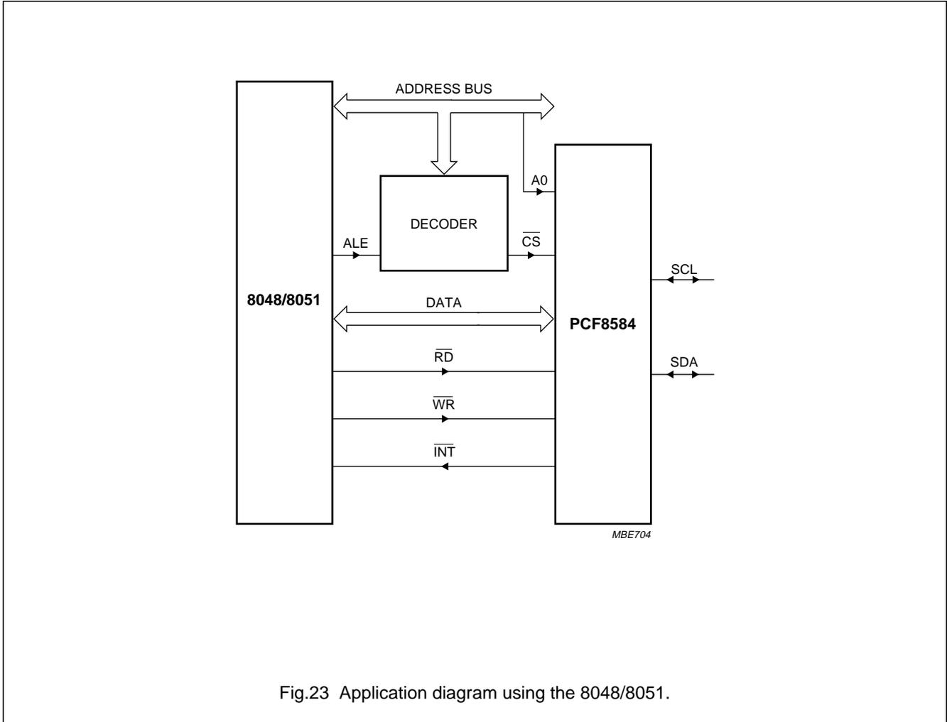
Fig.23 Application diagram using the 8048/8051.
