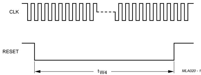
Fig.21 Reset timing.
