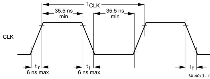
Fig.14 Clock input timing.
