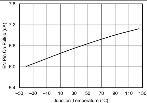
**Figure 17. EN Pin Pullup Current vs Temperature, EN = 1.5 V**
