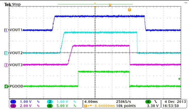
Figure 58. Automatic Power Sequencing, MODE = EN1 = EN2 = HIGH
