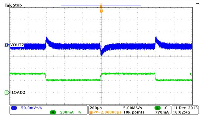
Figure 48. Buck2, Load Transient, 0.5 to 0.75 A SR = 0.25 A/µs
