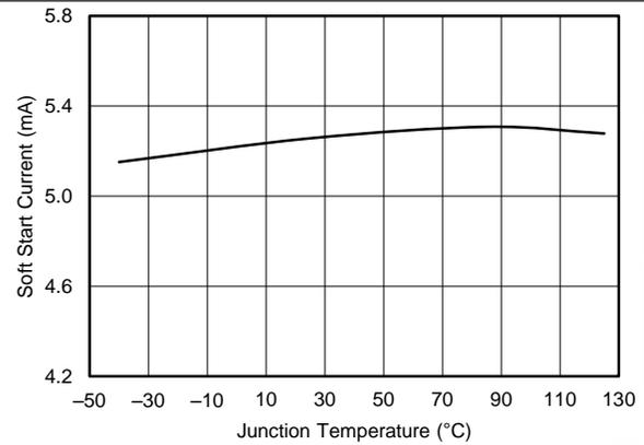
**Figure 20. SS Pin Charge Current vs Temperature**
