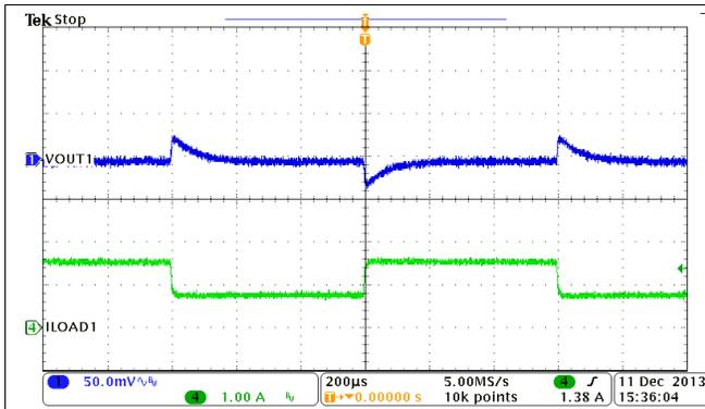
Figure 45. Buck1, Load Transient, 0.75 to 1.5 A SR = 0.25 A/µs
