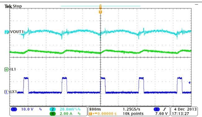
Figure 40. Buck1, Steady State Operation at Full Load
