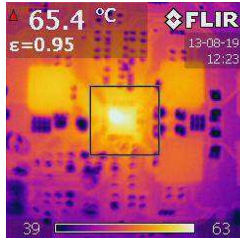
Operating at VIN = 12 V, VOUT1 = 1.2 V / 3 A, VOUT2 = 1.8 V / 1 A, VOUT3 = 3.3 V / 1 A,
