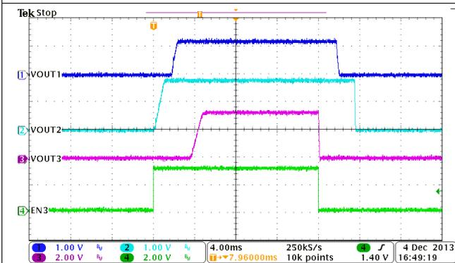
Figure 61. Automatic Power Sequencing, MODE = EN2 = HIGH, EN1 = LOW
