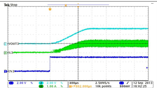
Figure 38. BUCK3, Soft-Start With Full Load
