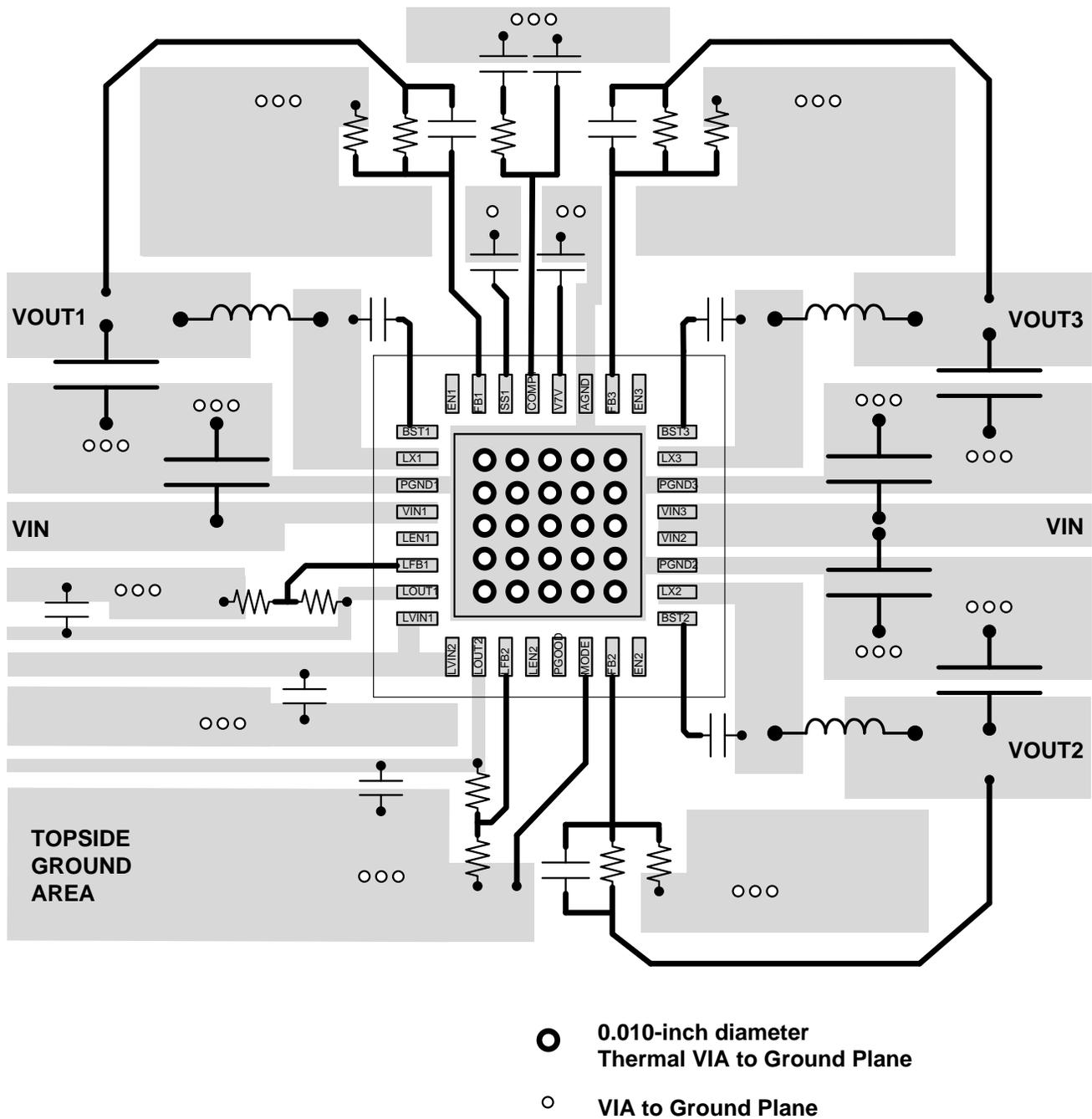
Figure 65. PCB Layout
