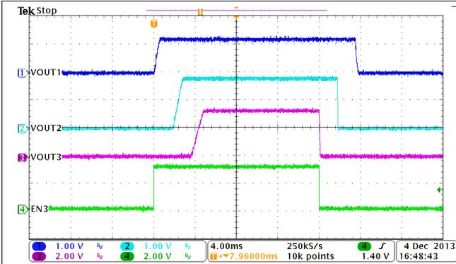
Figure 57. Automatic Power Sequencing, MODE = EN1 = EN2 = HIGH
