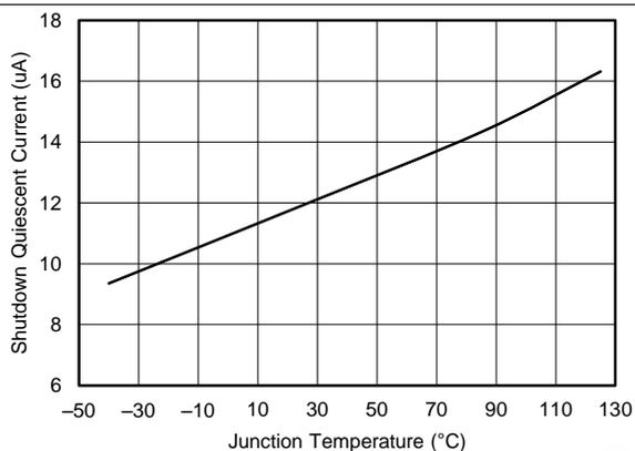
**Figure 15. Shutdown Quiescent Current vs Temperature**
