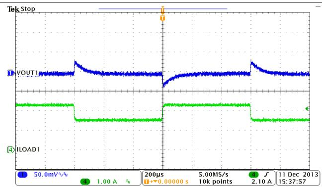
Figure 46. Buck1, Load Transient, 1.5 to 2.25 A SR = 0.25 A/µs
