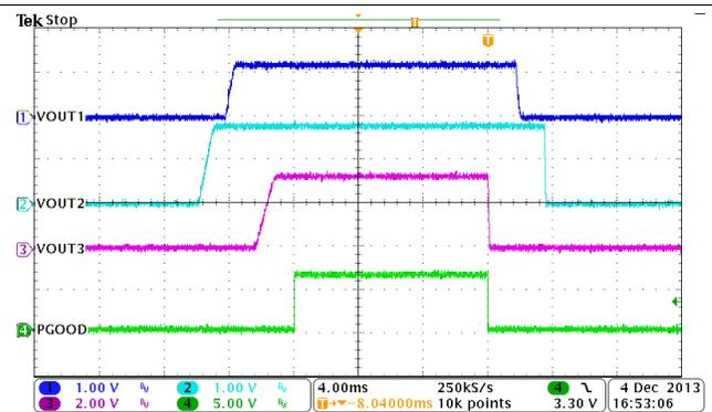
Figure 62. Automatic Power Sequencing, MODE = EN2 = HIGH, EN1 = LOW
