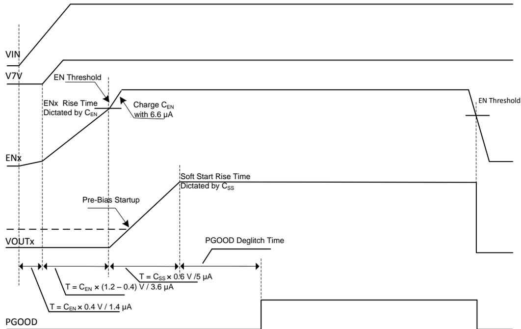
Figure 27. Startup Power Sequence
