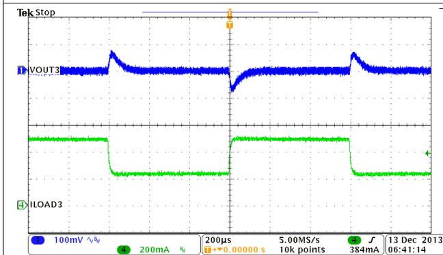
Figure 49. Buck3, Load Transient, 0.25 to 0.5 A SR = 0.25 A/µs
