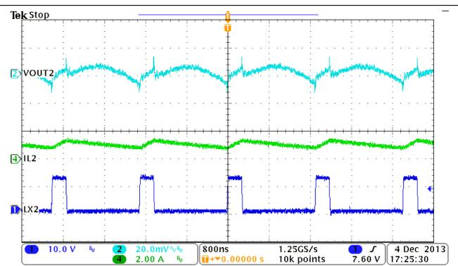
Figure 42. Buck2, Steady State Operation at Full Load
