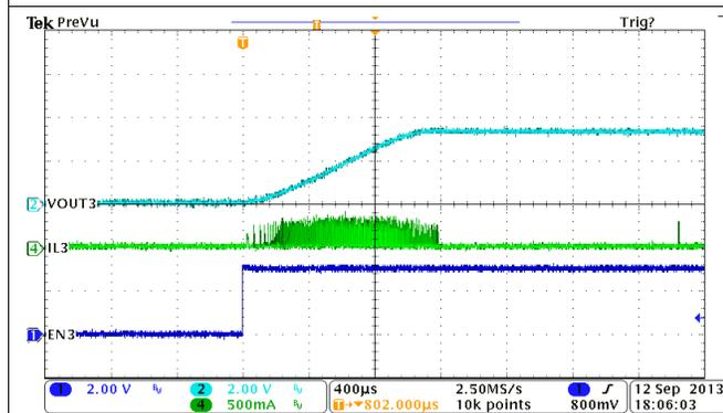
Figure 37. BUCK3, Soft-Start With No Load
