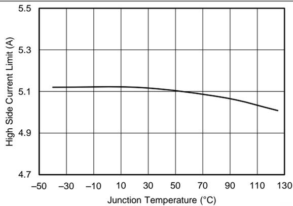
**Figure 21. Buck1 High-Side Current Limit vs Temperature**
