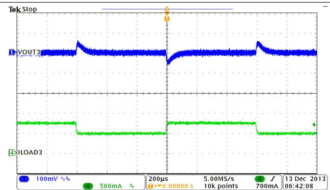
Figure 50. Buck3, Load Transient, 0.5 to 0.75 A SR = 0.25 A/µs
