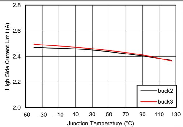
**Figure 22. Buck2, 3 High-Side Current Limit vs Temperature**
