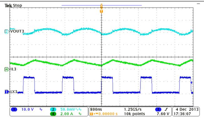
Figure 44. Buck3, Steady State Operation at Full Load
