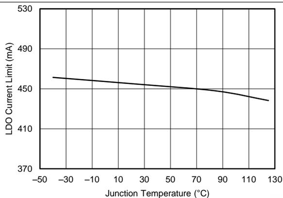
**Figure 23. LDO Current Limit vs Temperature**
