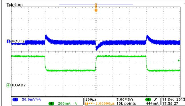
Figure 47. Buck2, Load Transient, 0.25 to 0.5 A SR = 0.25 A/µs
