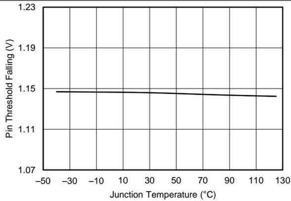
**Figure 19. EN Pin Threshold Falling vs Temperature**
