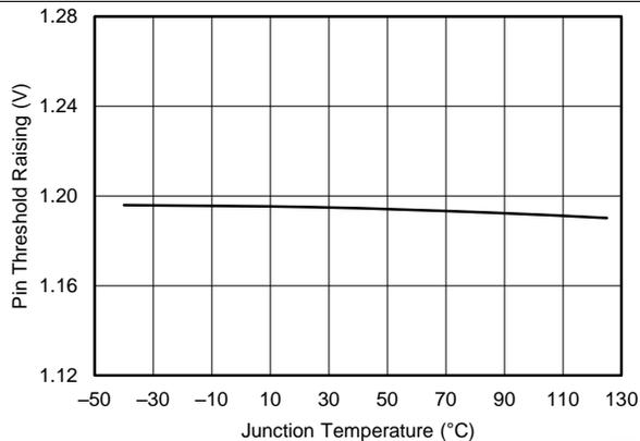
**Figure 18. EN Pin Threshold Rising vs Temperature**
