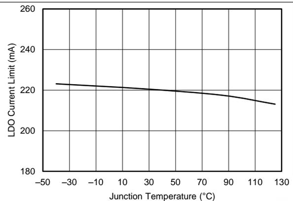
**Figure 24. LDO2 Current Limit vs Temperature**
