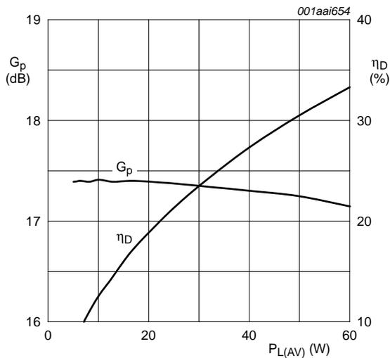
$V_{DS} = 30\text{ V}$ ;  $I_{Dq} = 1400\text{ mA}$ ;  $f = 1960\text{ MHz}$  ( $\pm 5\text{ MHz}$ ); carrier spacing 10 MHz.
