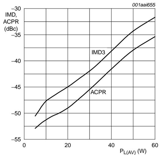
$V_{DS} = 30\text{ V}$ ;  $I_{Dq} = 1400\text{ mA}$ ;  $f = 1960\text{ MHz}$  ( $\pm 5\text{ MHz}$ ); carrier spacing 10 MHz.
