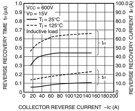
**SWITCHING RECOVERY LOSS CHARACTERISTICS (TYPICAL)**
