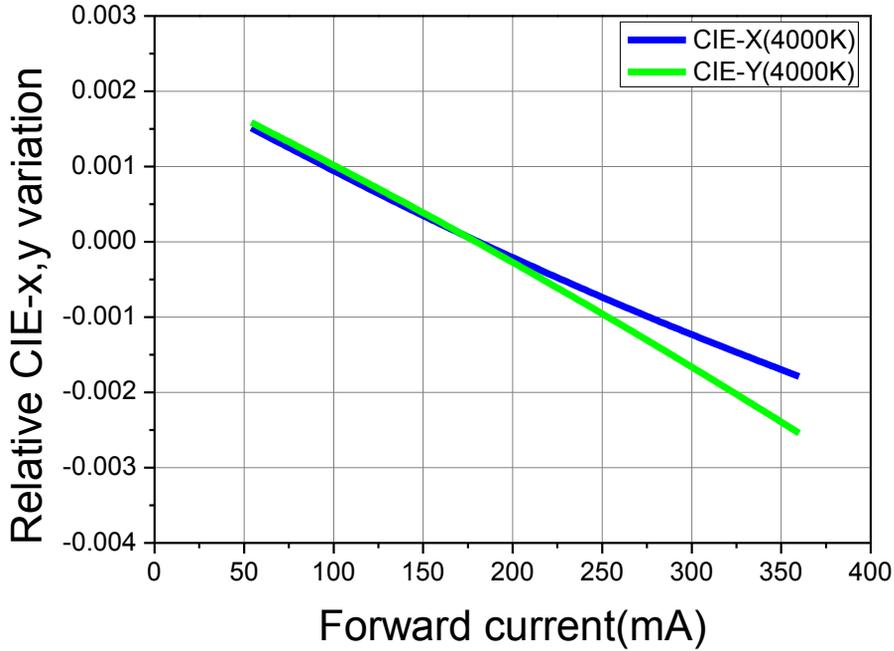
**Fig 17. Forward current vs. CIE x,y Shift,  $T_j=85^{\circ}\text{C}$  (CRI90, 3000K)**
