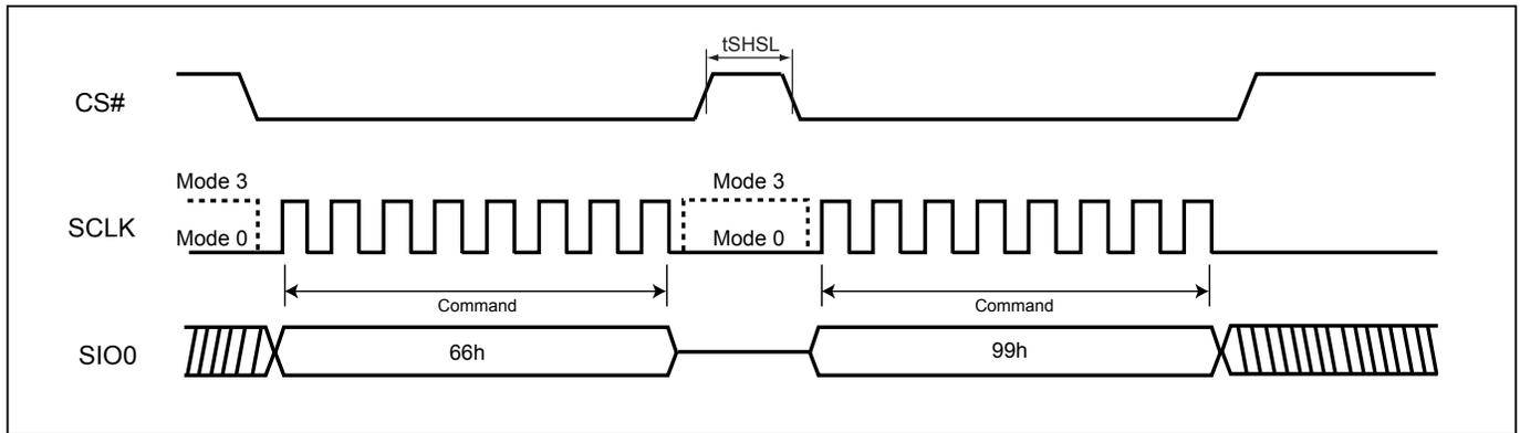
**Figure 99. Reset Sequence (QPI mode)**
