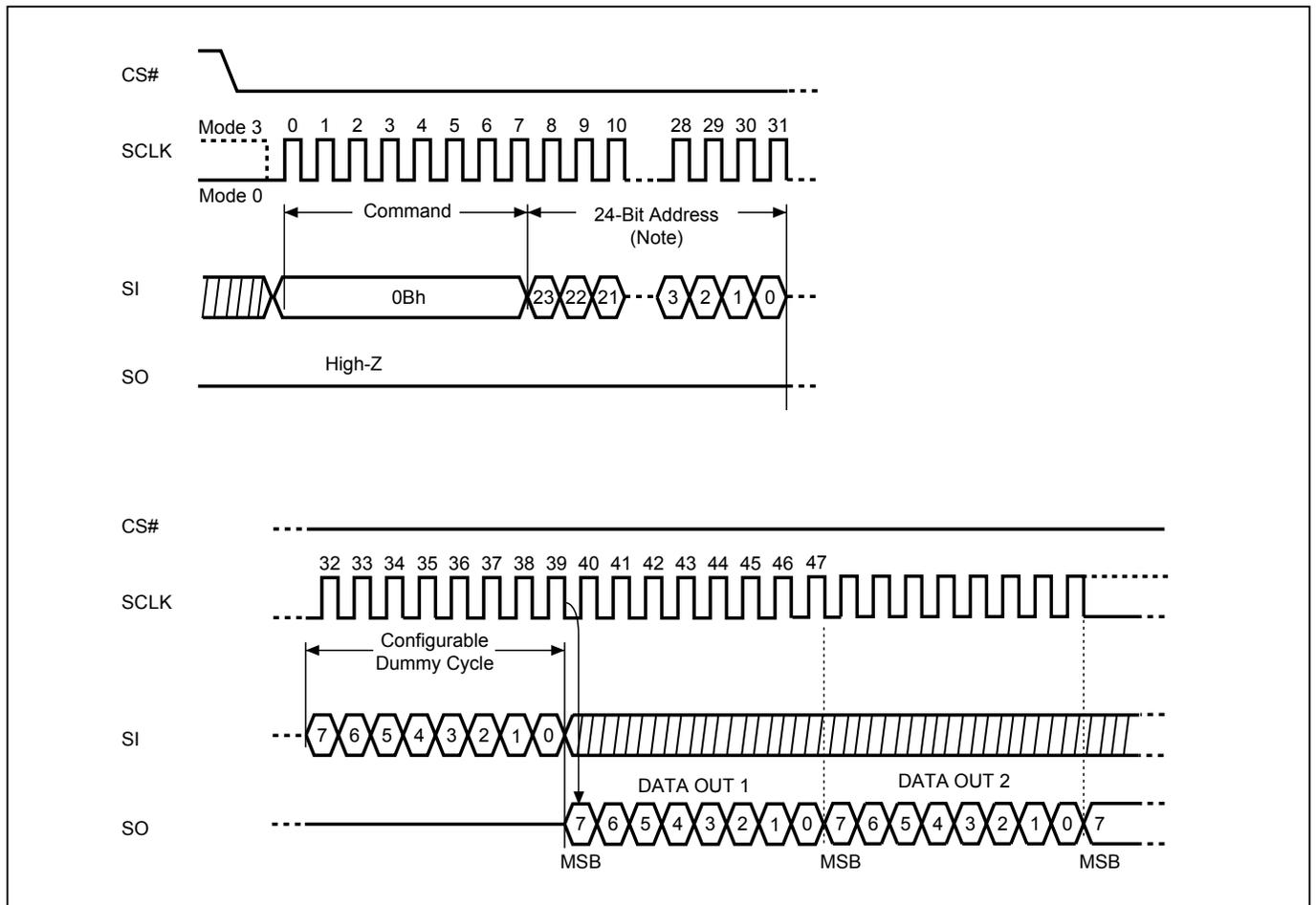
Note: Please note the address cycles above are based on 3-byte address mode. For 4-byte address mode, the address cycles will be increased.
