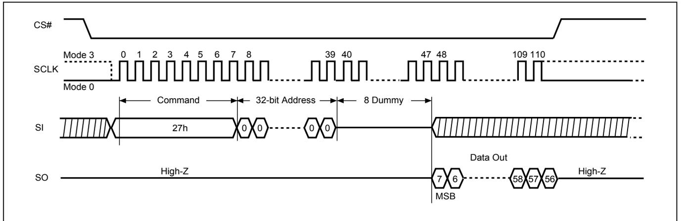
**Figure 91. Write Password Register (WRPASS) Sequence**
