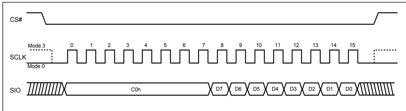
**Figure 62. Burst Read (QPI Mode)**
