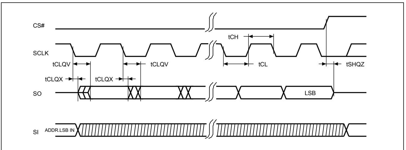
**Figure 4. Output Timing (DTR mode)**
