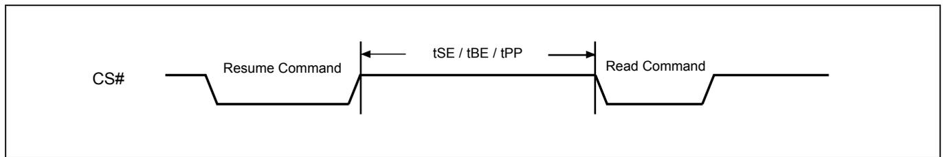
**Figure 96. Resume to Suspend Latency**
