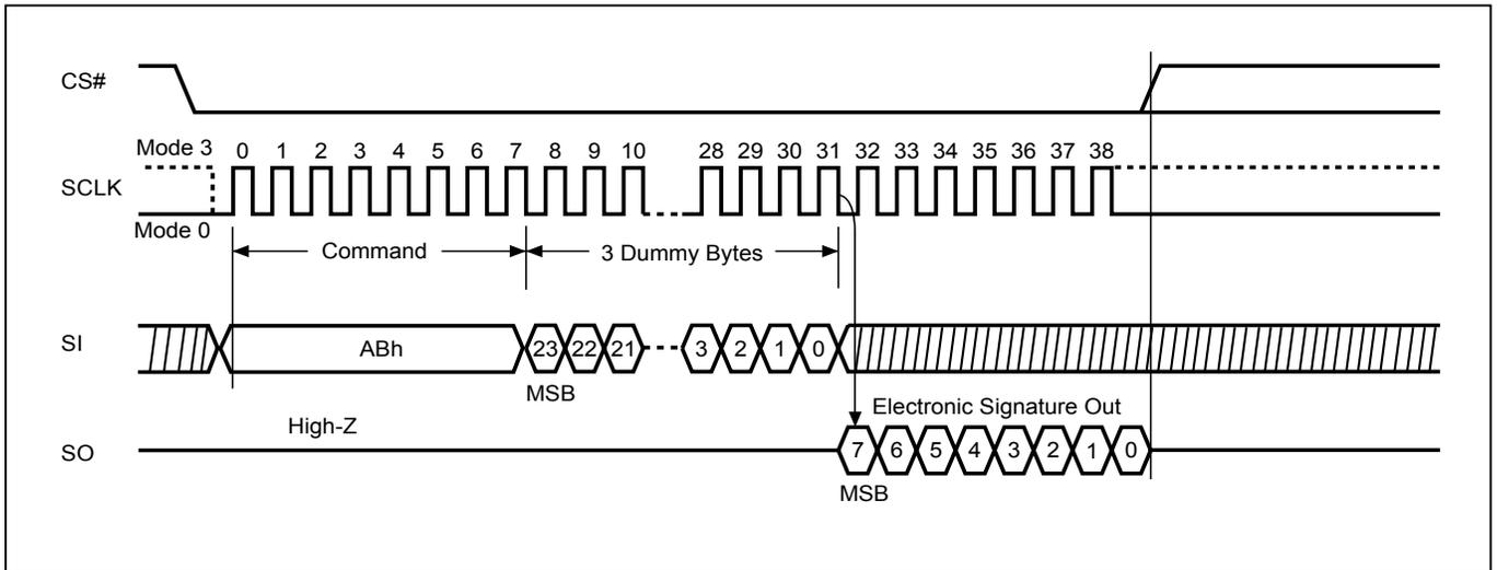
**Figure 18. Read Electronic Signature (RES) Sequence (QPI Mode)**
