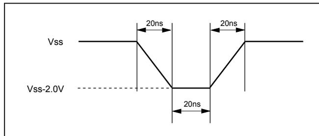
**Figure 103. Maximum Positive Overshoot Waveform**
