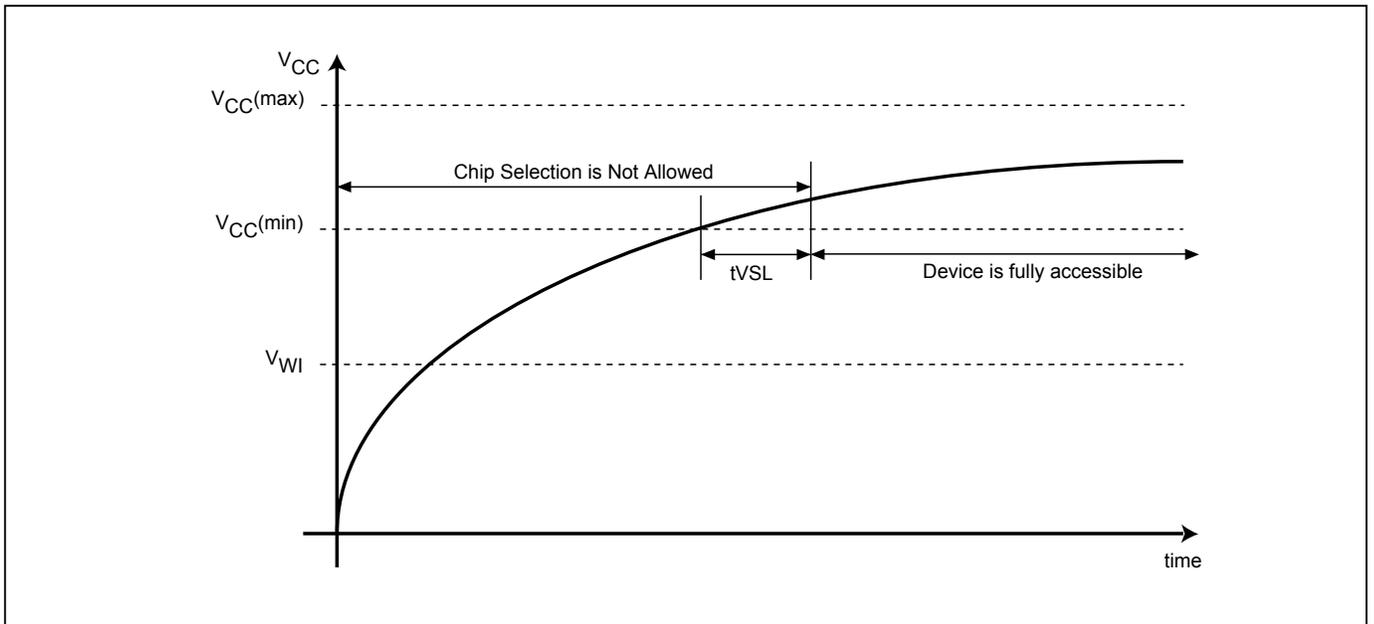
**Figure 110. Power Up/Down and Voltage Drop**
