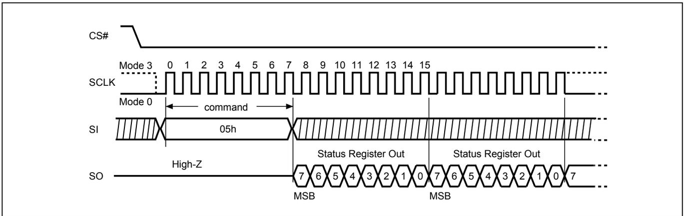
**Figure 21. Read Status Register (RDSR) Sequence (QPI Mode)**
