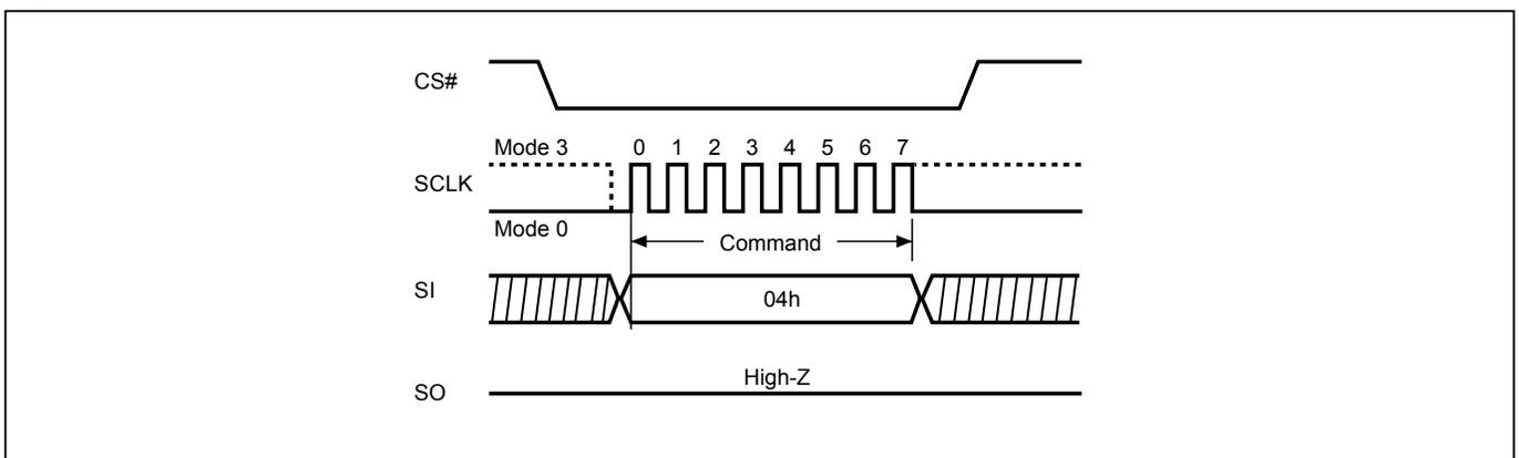
**Figure 15. Write Disable (WRDI) Sequence (QPI Mode)**
