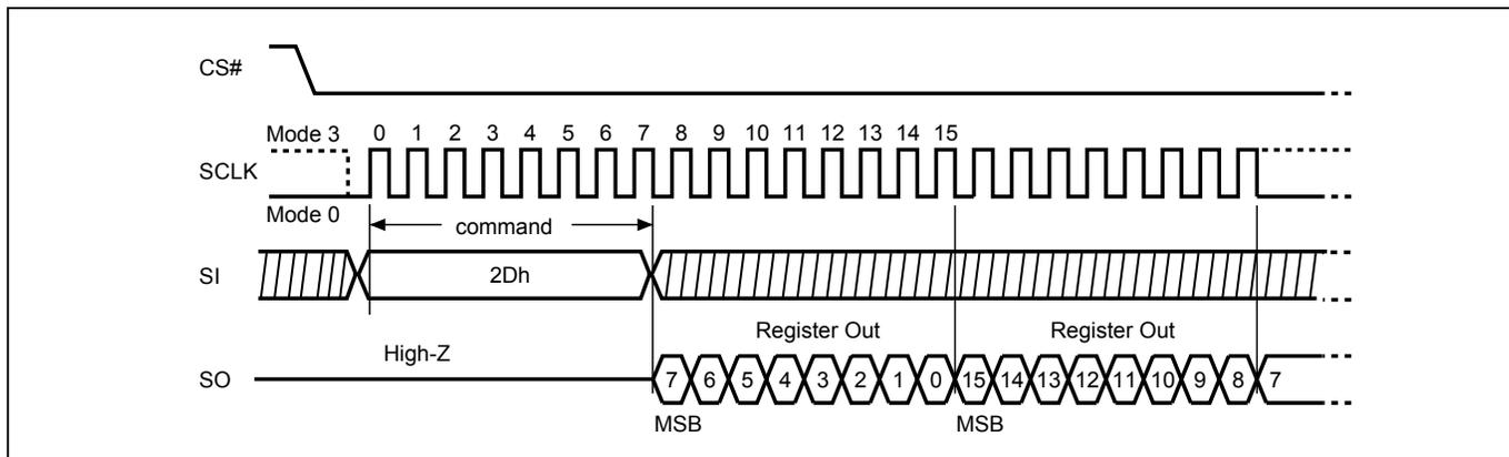
**Figure 84. Write Lock Register (WRLR) Sequence (SPI Mode)**
