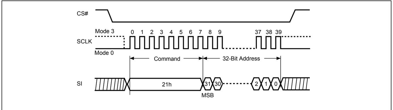
**Figure 53. Block Erase 32KB (BE32K4B) Sequence (SPI Mode)**
