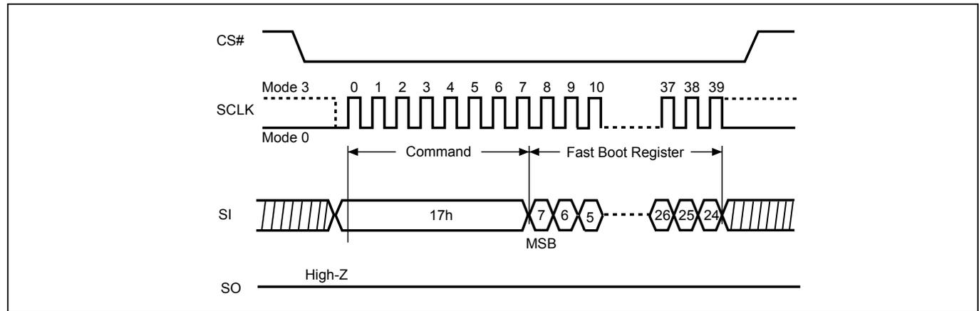
**Figure 67. Erase Fast Boot Register (ESFBR) Sequence**
