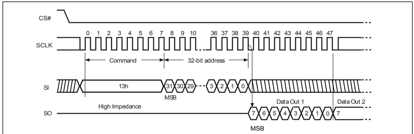
**Figure 47. Read Data Bytes at Higher Speed using 4 Byte Address Sequence (FASTREAD4B)**
