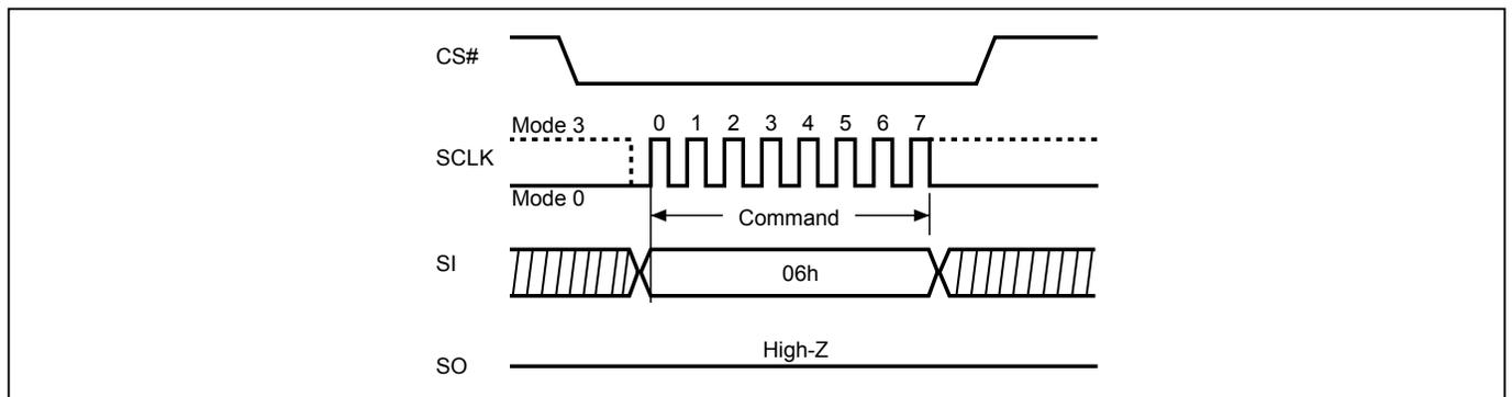
**Figure 13. Write Enable (WREN) Sequence (QPI Mode)**
