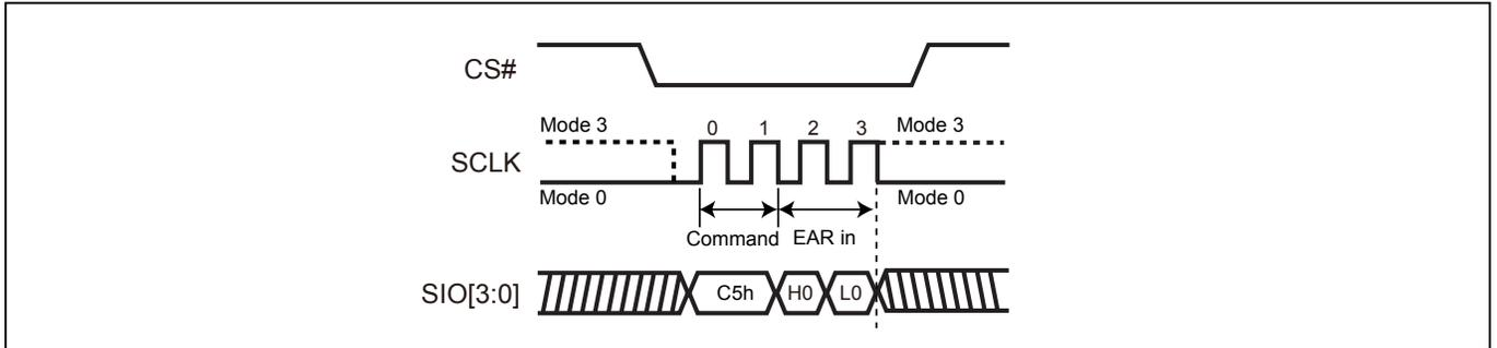
**Figure 8. Read EAR (RDEAR) Sequence (SPI Mode)**
