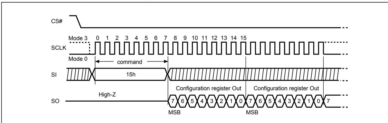
**Figure 23. Read Configuration Register (RDCR) Sequence (QPI Mode)**
