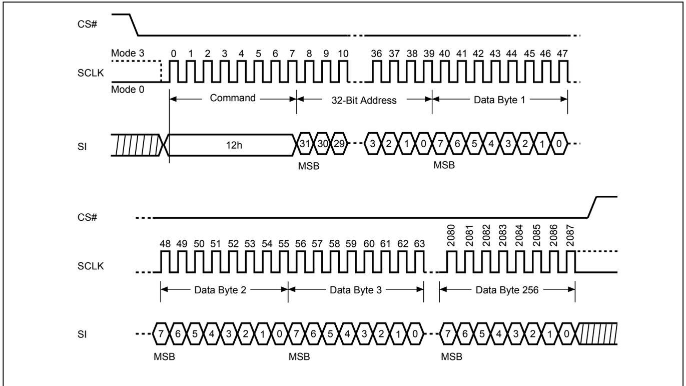
**Figure 56. 4 x I/O Page Program (4PP4B) Sequence (SPI Mode only)**
