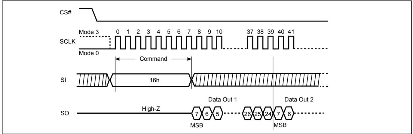
**Figure 66. Write Fast Boot Register (WRFBR) Sequence**
