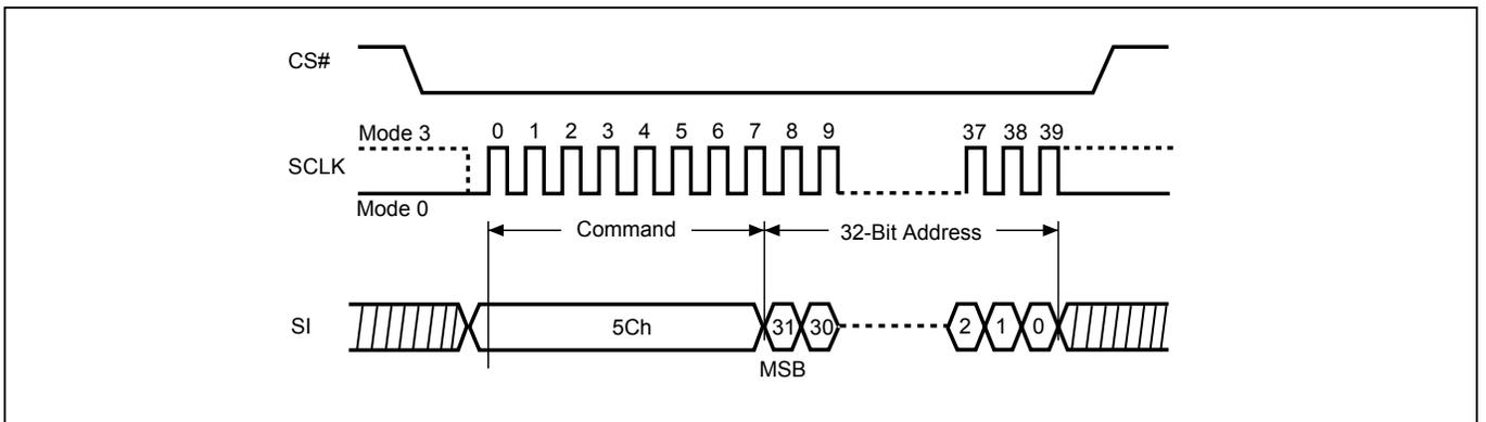
**Figure 54. Block Erase (BE4B) Sequence (SPI Mode)**
