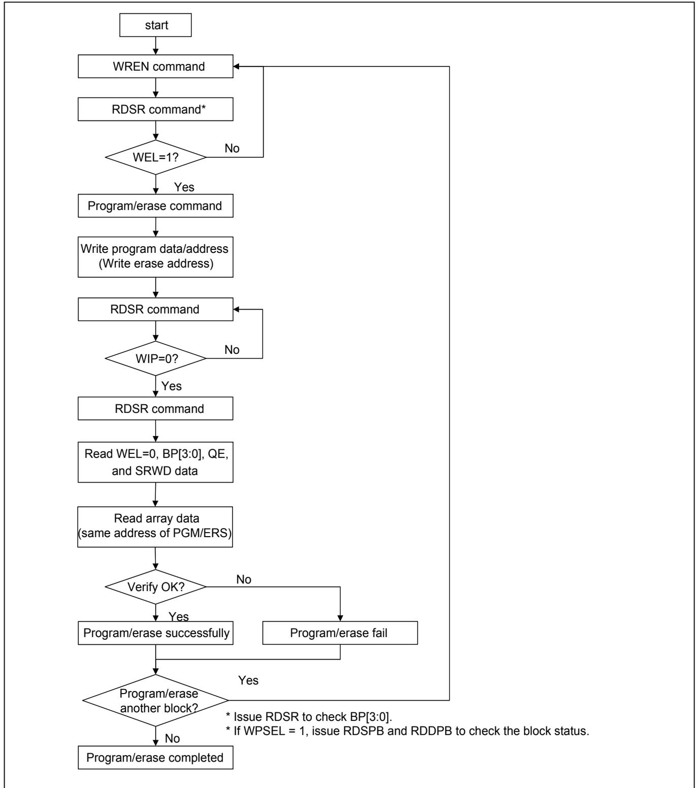
**Figure 25. Program/Erase flow without read array data (read P\_FAIL/E\_FAIL flag)**
