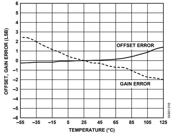
Figure 20. Offset and Gain Error vs. Temperature
