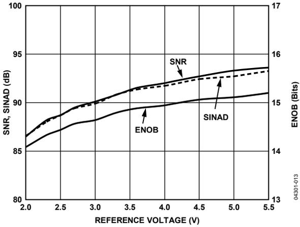
Figure 14. SNR, SINAD, and ENOB vs. Reference Voltage
