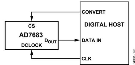
Figure 26. Connection Diagram
