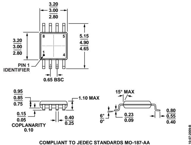
Figure 27. 8-Lead Mini Small Outline Package [MSOP] (RM-8)
