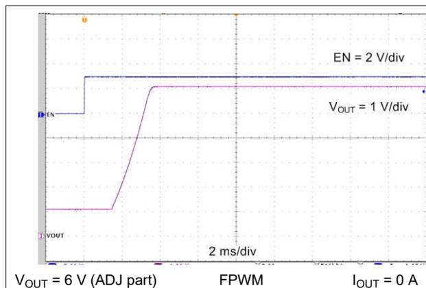
**Figure 9-31. Start-Up Waveform**
