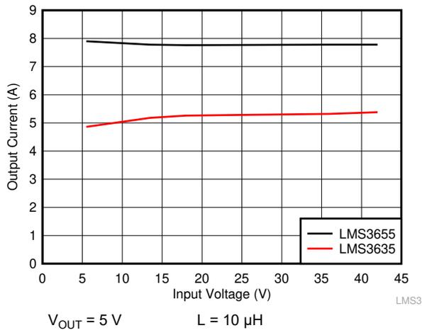
**Figure 9-13. Output Current Level Limit Before Overcurrent Protection**
