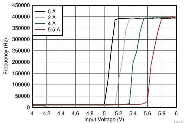
**Figure 8-11. Frequency Dropout Characteristics ( $V_{OUT} = 5\text{ V}$ )**
