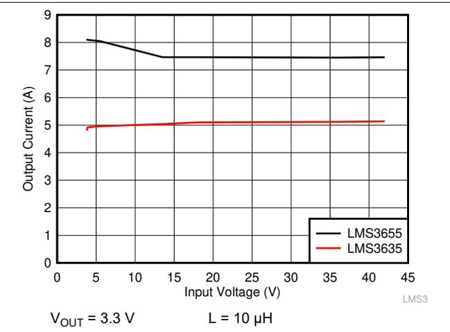
**Figure 9-26. Output Current Level for Overcurrent Protection Trip**
