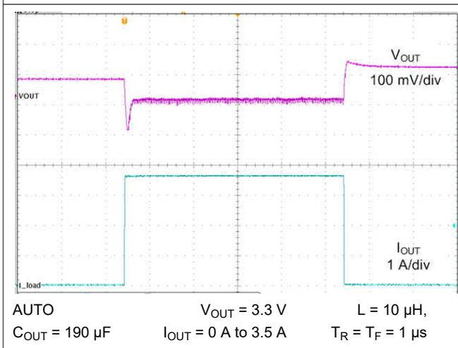
**Figure 9-27. Load Transient**
