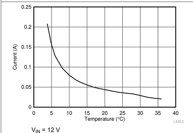
**Figure 7-5. Short Circuit Average Input Current for LMS3635-Q1**
