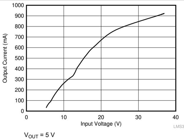
Figure 9-9. Load Current for PFM-to-PWM Transition
