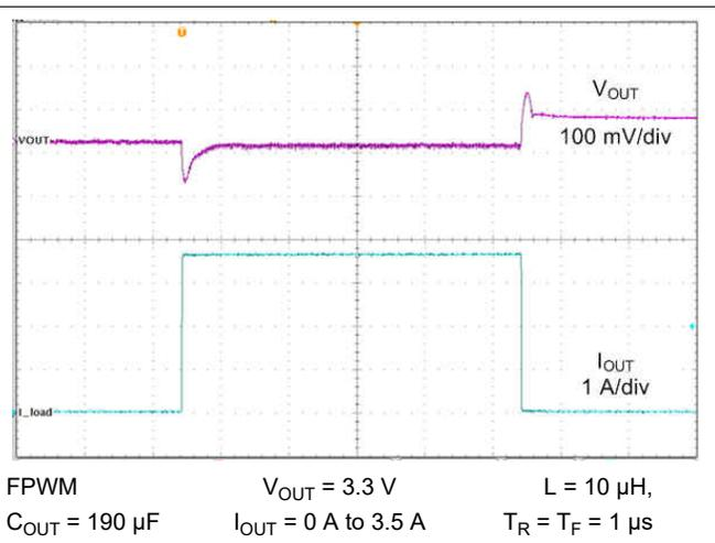
**Figure 9-28. Load Transient**
