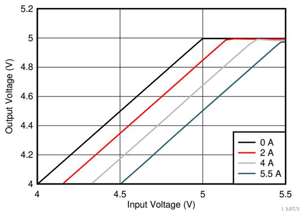
**Figure 8-10. Overall Dropout Characteristics ( $V_{OUT} = 5\text{ V}$ )**
