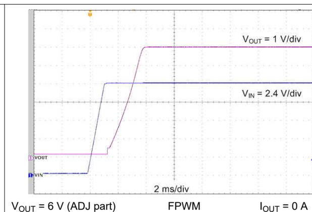
**Figure 9-32. Start-Up Waveform (EN Tied to VIN)**
