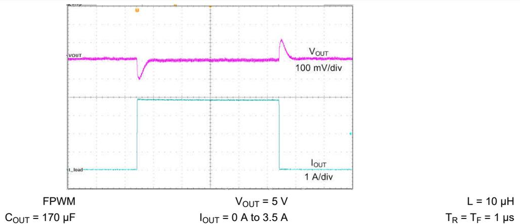
**Figure 9-15. Load Transient**
