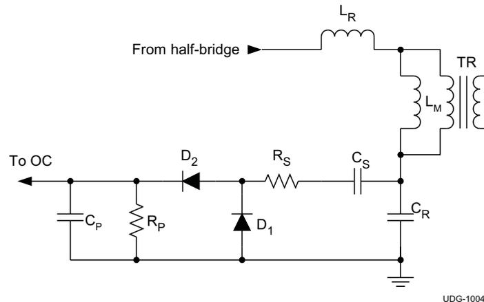
**Figure 20. Current Sensing for LLC Resonant Converter**
