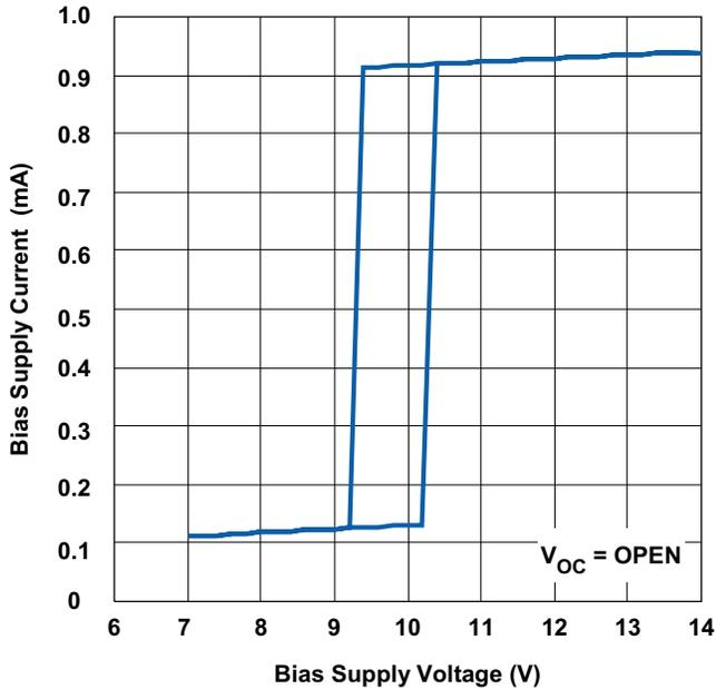
Figure 1. Bias Supply Current vs. Bias Supply Voltage
