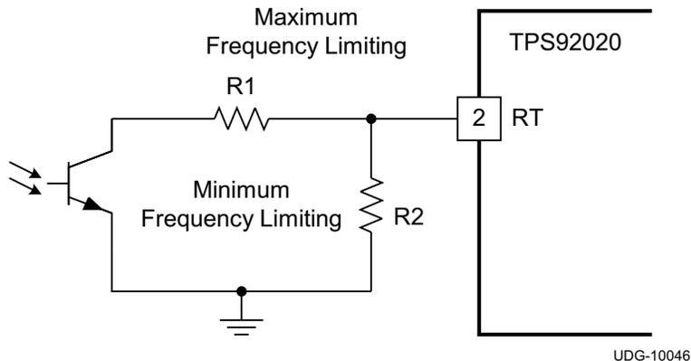
Figure 18. Maximum and Minimum Frequency Setting for TPS92020
