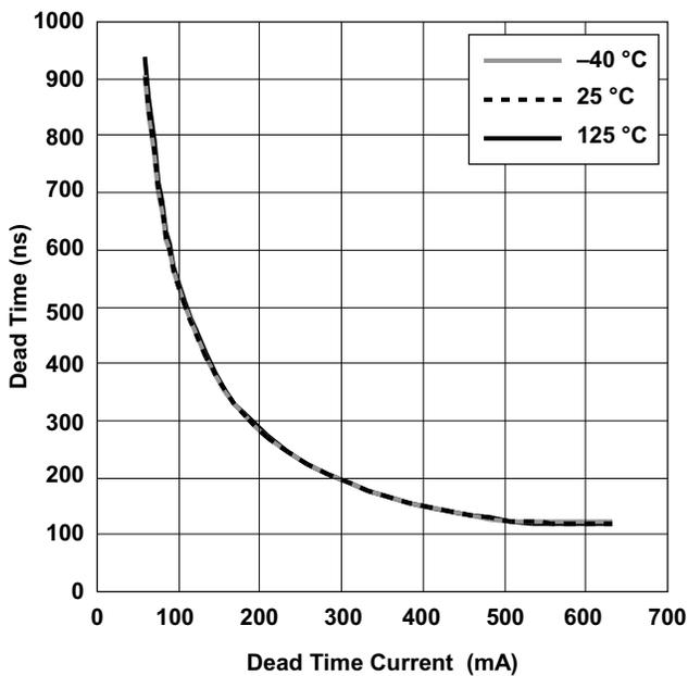
Figure 3. Dead Time vs. Dead Time Current
