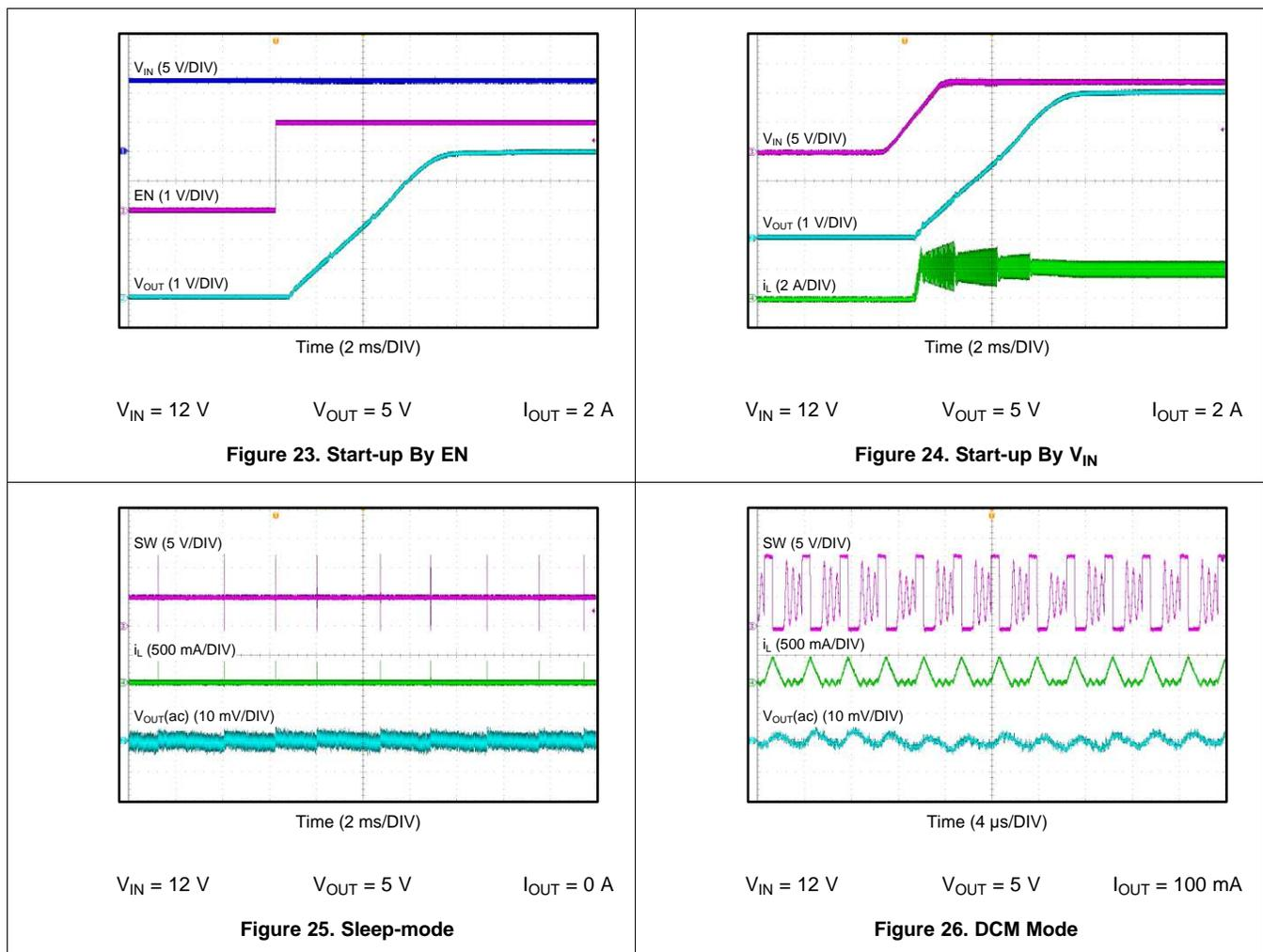
Unless otherwise specified the following conditions apply:  $V_{IN} = 12\text{ V}$ ,  $f_{SW} = 300\text{ kHz}$ ,  $L = 6.5\text{ }\mu\text{H}$ ,  $C_{OUT} = 47\text{ }\mu\text{F} \times 4$ ,  $T_A = 25\text{ }^\circ\text{C}$
