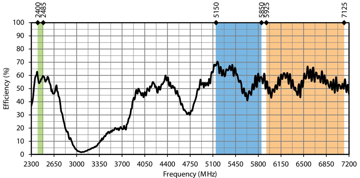
Figure 8. W63WS1 Series Antenna Radiation Efficiency, Straight
