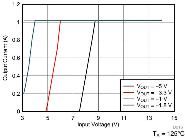
Figure 39. Maximum Output Current vs Input Voltage
