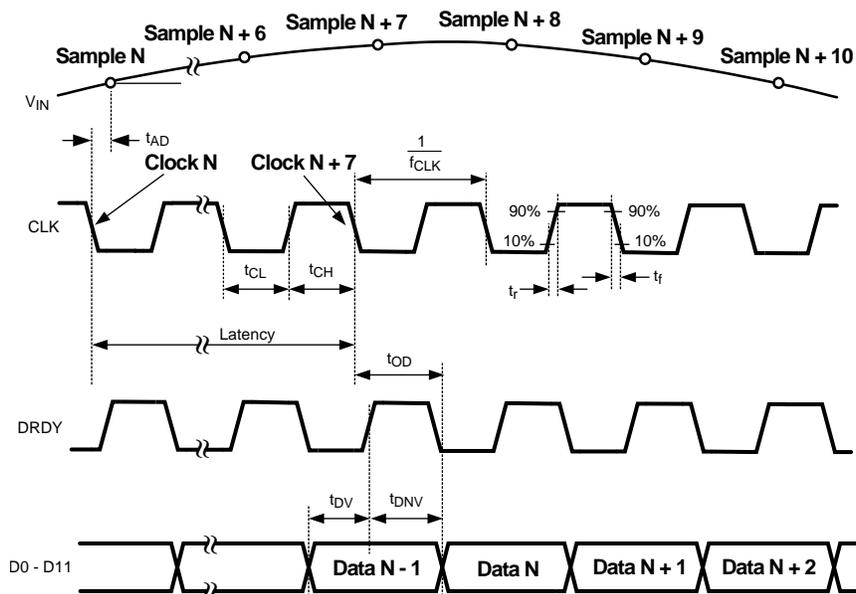
Figure 1. Output Timing
