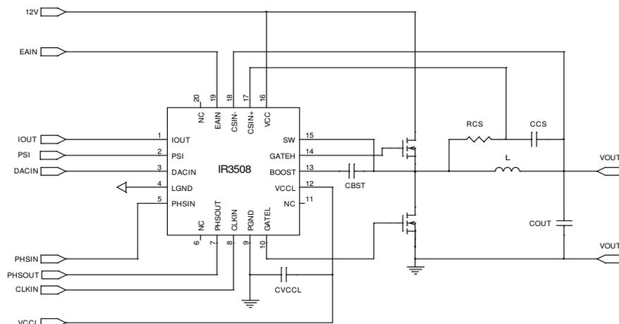
Figure 1 Application Circuit
