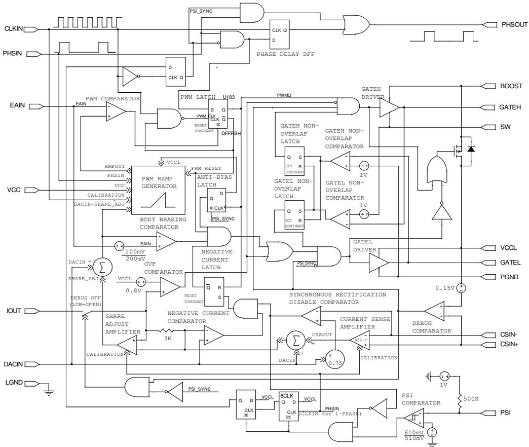
Figure 5: Block diagram
