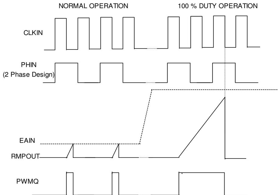
Figure 6: PWM Operation during normal and 100 % duty mode.
