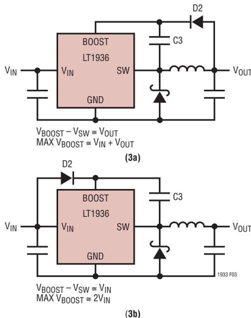
Figure 3. Two Circuits for Generating the Boost Voltage
