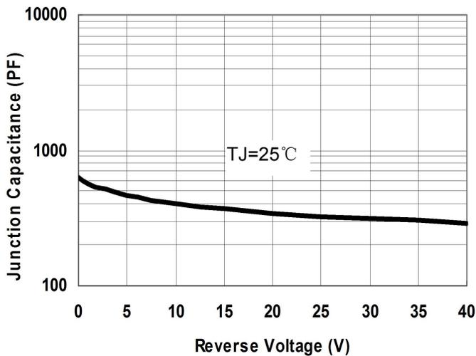
Fig.1-Typical Junction Capacitance
