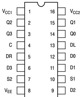
Pin assignment is for Dual-in-Line Package.
