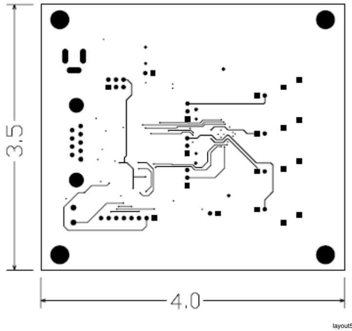
FIGURE 6. LP3906EVB Bottom layer Plot
