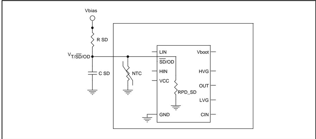
RPD\_SD: equivalent value as result of resistances of three drivers in parallel.
