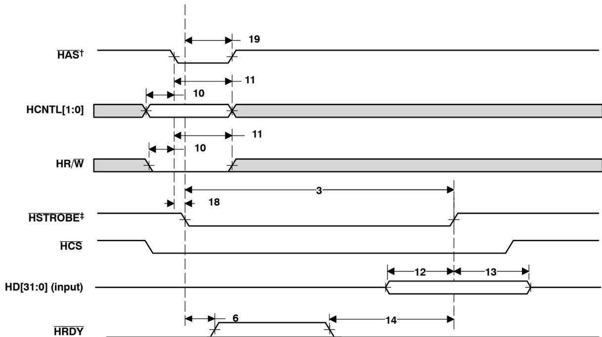
† For correct operation, strobe the **HAS** signal only once per **HSTROBE** active cycle.
