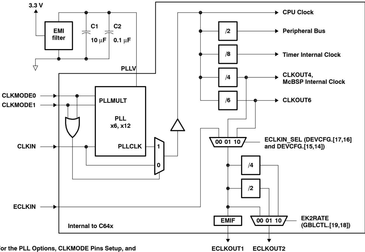
(For the PLL Options, CLKMODE Pins Setup, and PLL Clock Frequency Ranges, see Table 31.)
