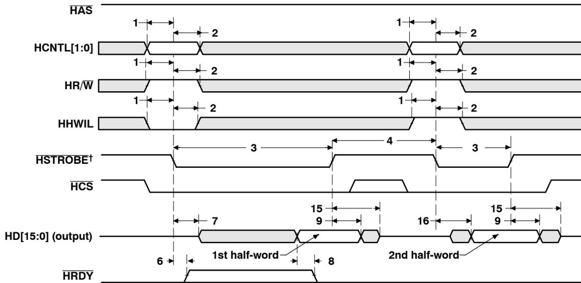
† HSTROBE refers to the following logical operation on HCS, HDST1, and HDS2:  $[\text{NOT}(\text{HDST1 XOR HDS2})] \text{ OR HCS}$ .
