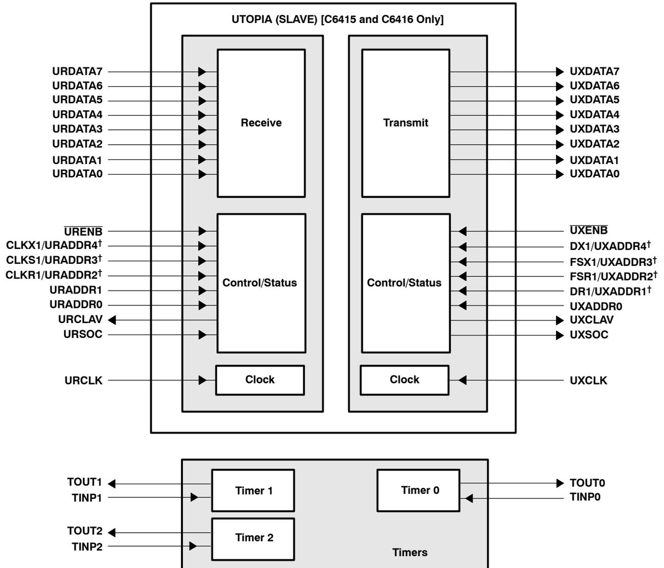
† For the C6415 and C6416 devices, these UTOPIA pins are muxed with the McBSP1 peripheral. By default, these signals function as McBSP1. For more details on these muxed pins, see the Device Configurations section of this data sheet.
