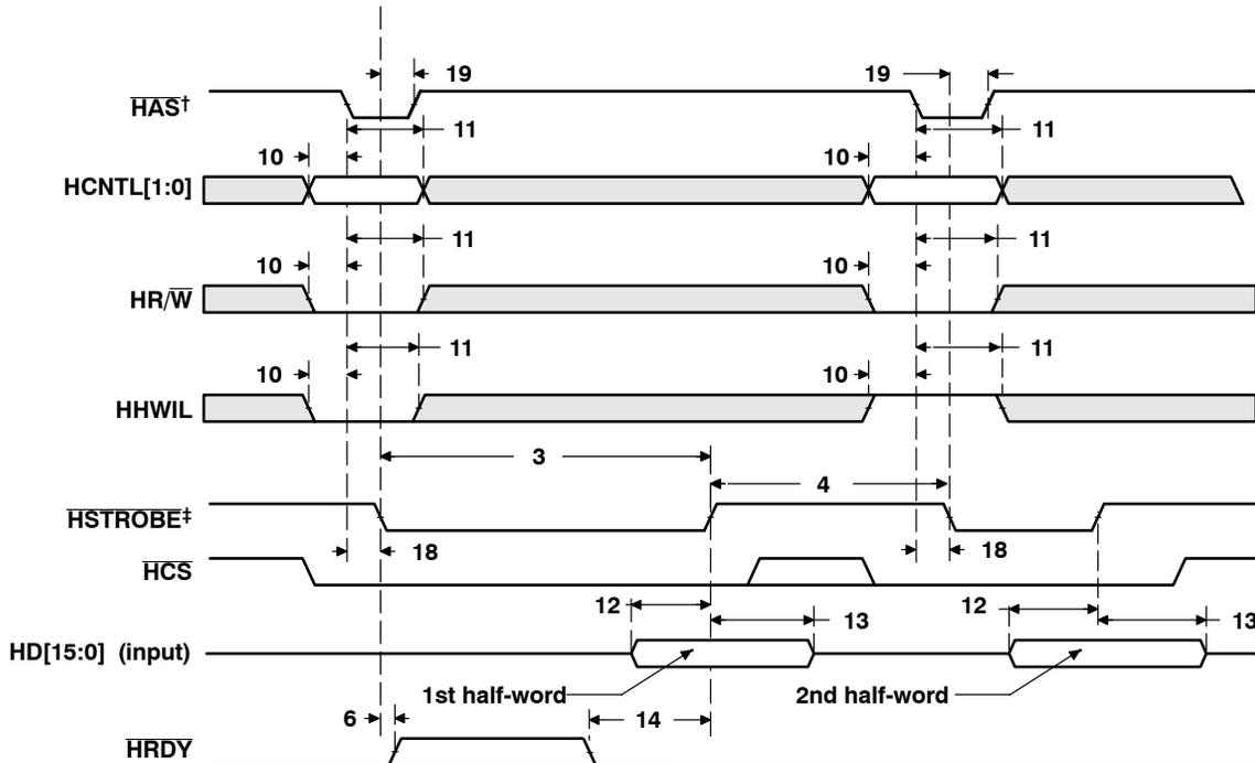
† For correct operation, strobe the HAS signal only once per HSTROBE active cycle.
