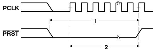
Figure 48. PCI Reset ( $\overline{PRST}$ ) Timing
