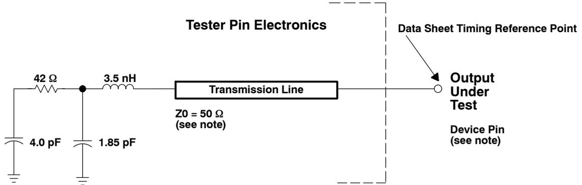
NOTE: The data sheet provides timing at the device pin. For output timing analysis, the tester pin electronics and its transmission line effects must be taken into account. A transmission line with a delay of 2 ns or longer can be used to produce the desired transmission line effect. The transmission line is intended as a load only. It is not necessary to add or subtract the transmission line delay (2 ns or longer) from the data sheet timings.
