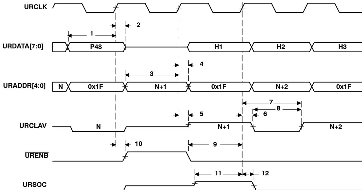
† The UTOPIA Slave module has signals that are middle-level signals indicating a high-impedance state (i.e., the URCLAV and URSOC signals).
