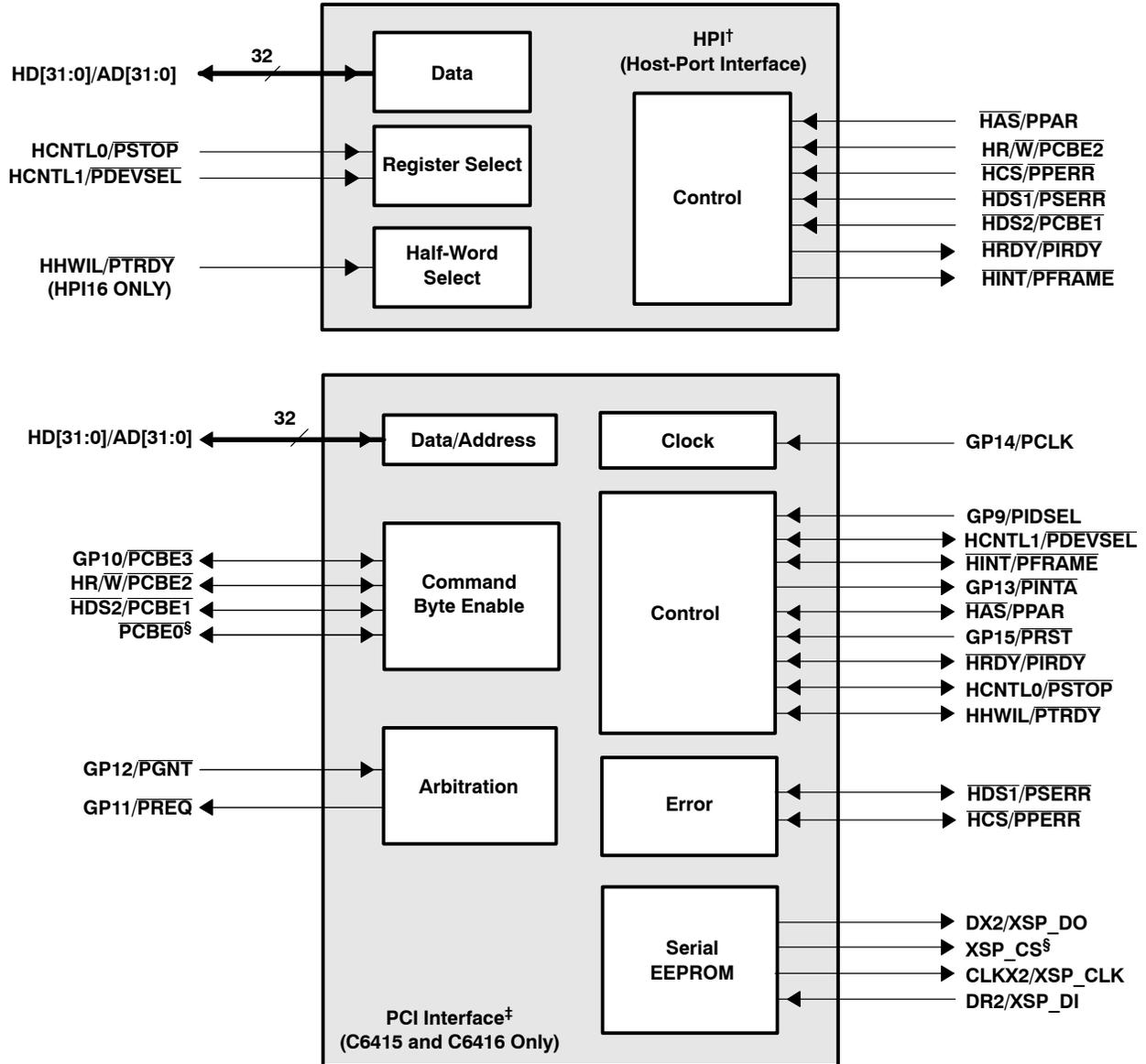
† For the C6415 and C6416 devices, these HPI pins are muxed with the PCI peripheral. By default, these signals function as HPI. For more details on these muxed pins, see the Device Configurations section of this data sheet. For the C6414 device, these HPI pins are *not* muxed; the C6414 device does *not* support the PCI peripheral.
