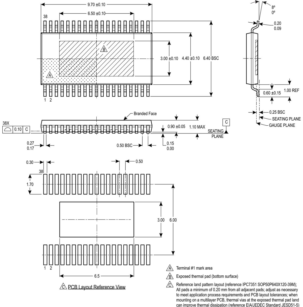
Figure 10: Package LV, 38-Pin eTSSOP
