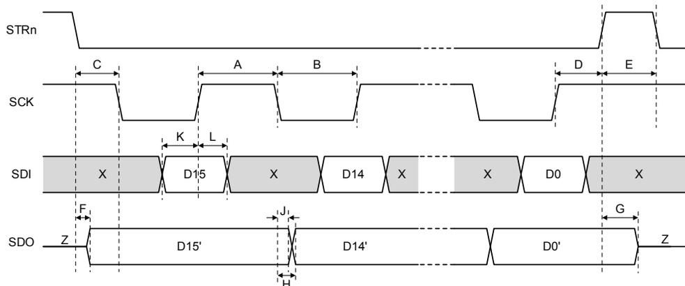
**Figure 1: Serial Interface Timing**
