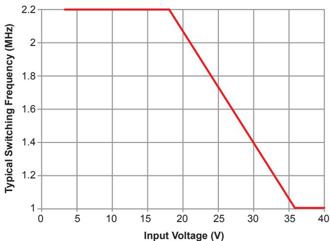
Figure 7: Typical Switching Frequency versus Input Voltage
