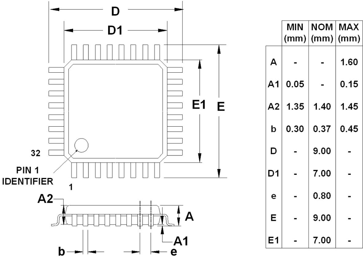
Figure 4.4. LQFP-32 Package Drawing
