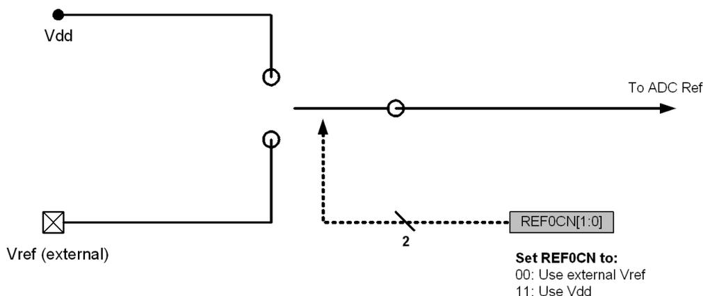
**Figure 7.1. Voltage Reference Functional Block Diagram**
