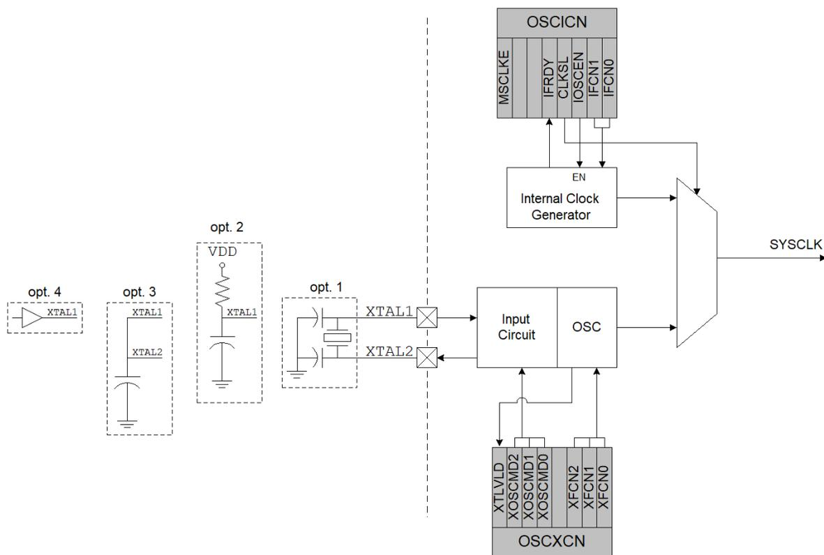
**Figure 13.1. Oscillator Diagram**
