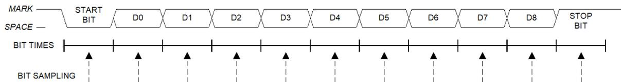
Figure 16.6. UART Modes 2 and 3 Timing Diagram
