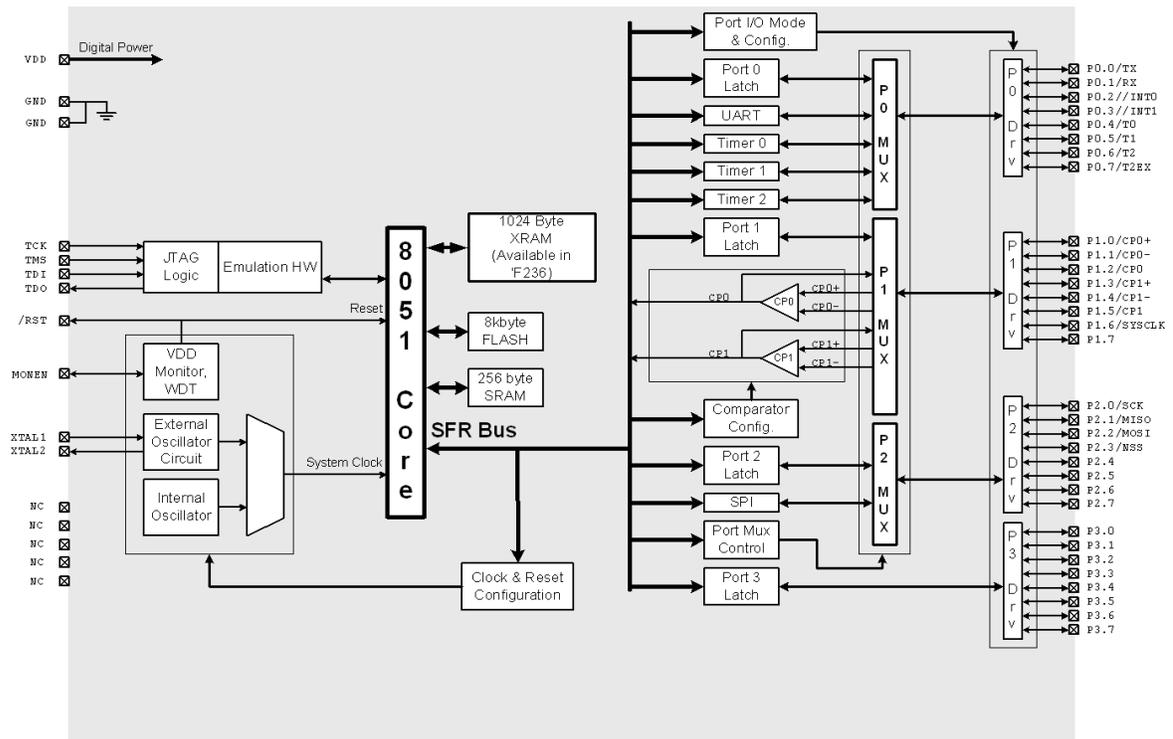
Figure 1.3. C8051F230 and C8051F236 Block Diagram (48 TQFP)
