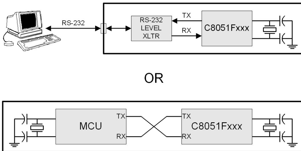
**Figure 16.5. UART Modes 1, 2, and 3 Interconnect Diagram**
