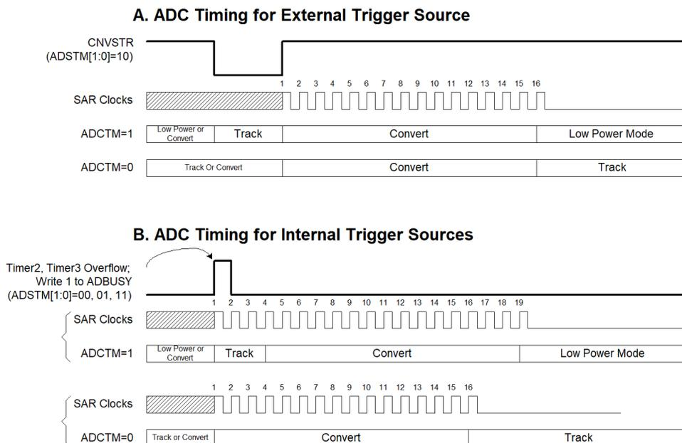
**Figure 6.2. 12-Bit ADC Track and Conversion Example Timing**
