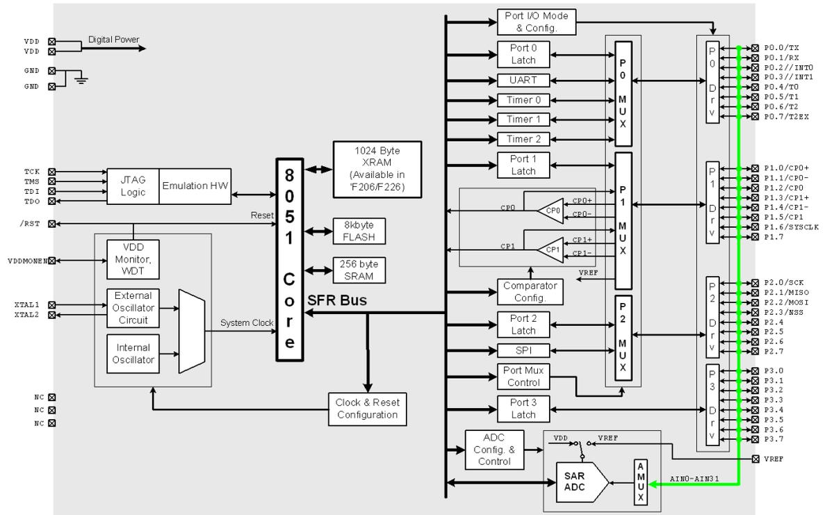
Figure 1.1. C8051F206, C8051F220 and C8051F226 Block Diagram (48 TQFP)
