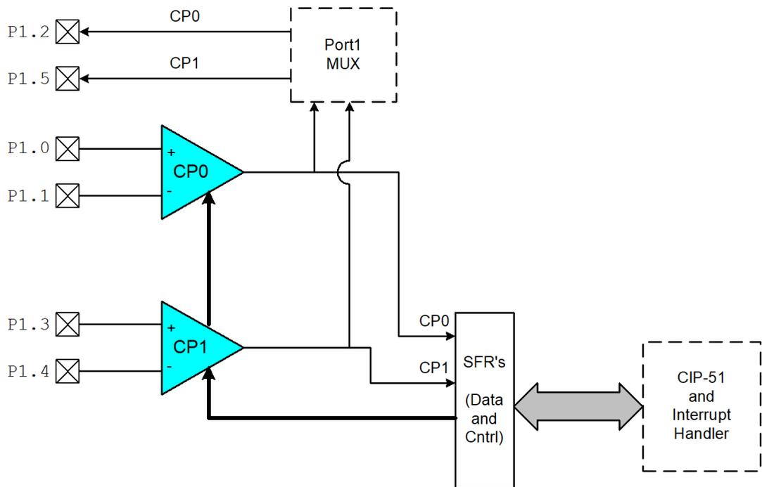
Figure 1.11. Comparator Diagram
