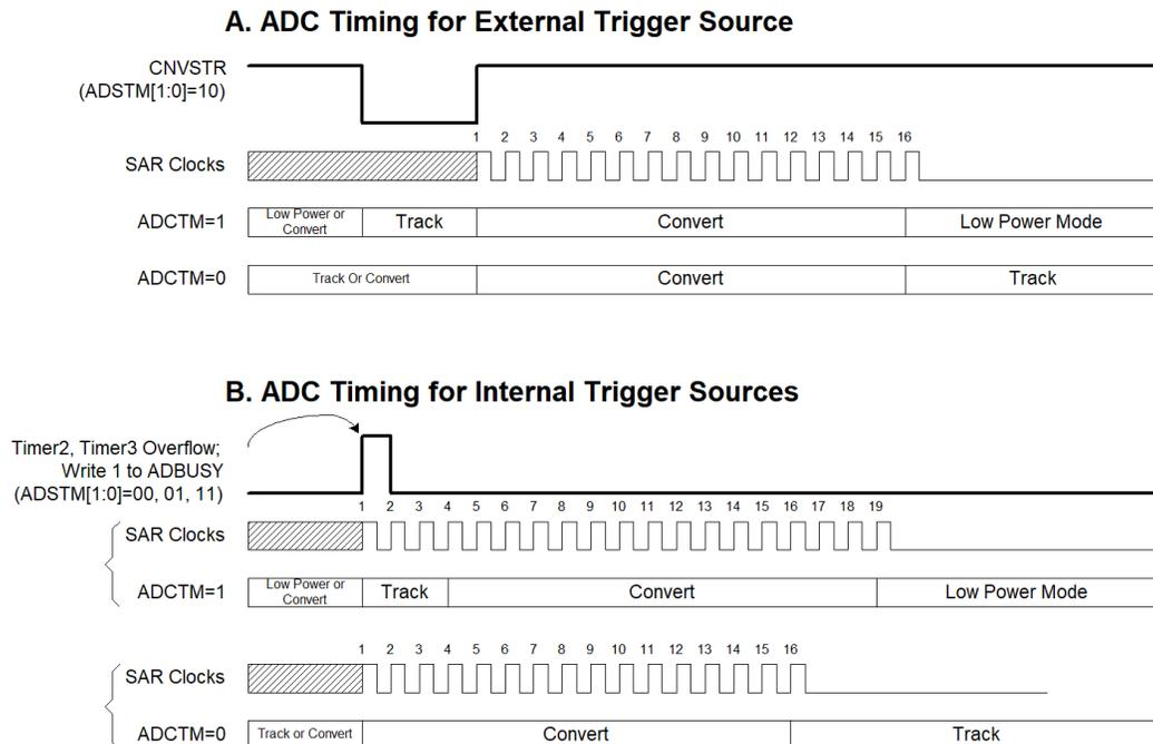
**Figure 5.2. 12-Bit ADC Track and Conversion Example Timing**
